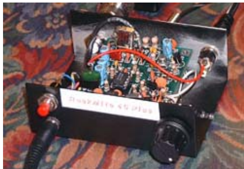
Rock-Mite 40 meter QRP transceiver.
