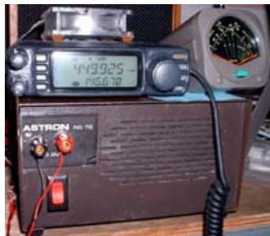
Node 4214 radio equipment. The Yaesu FT-7100 has an extra cooling fan on top.
