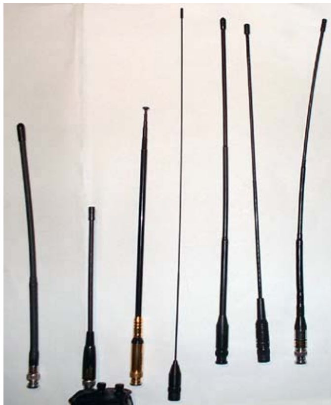
A selection of ducks and whips. Left to right: base loaded monoband duck, IC-Z1A stock antenna, generic half-wave telescopic, Pryme RD-98, Opek HR-12, Diamond RH77CA, TSC-2301.
