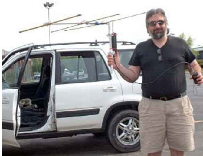
Mike, N2HTT shows the Yagi based on steel measuring-tape that he used to find the fox.
