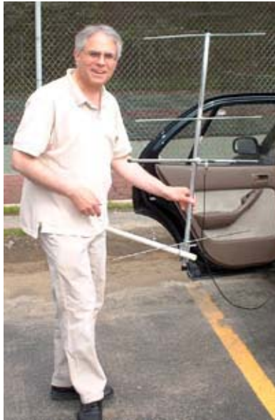
Karl, N2KZ shows the 161 MHz broadcast auxiliary antenna he adapted for the 2 meter foxhunt.
