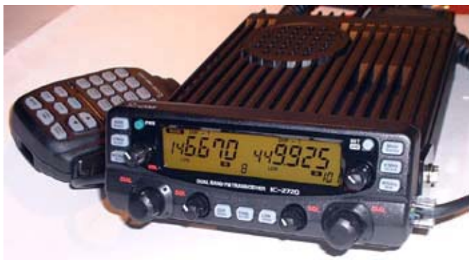
Icom's IC-2720H dual-band FM transceiver with the control head mounted to the transceiver body.
