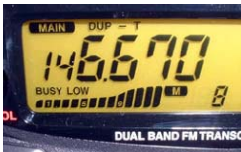
Close-up of left half of IC-2720H LCD display showing the 7-level S-meter.
