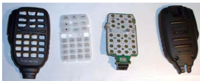
Disassembled HM-133 microphone. The hole for the electret microphone in the rubber molding may need to be enlarged to align with the matching hole in the front of the case.
