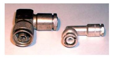
Right Angle Type N (left) and BNC connector (right) for coaxial cable. Paul Neill was involved in both designs.
