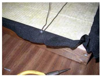
Construction of acoustic absorption panels as designed by WB2HNA. The mineral fiber material is covered with speaker grille cloth and set in a wood frame.
