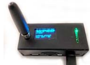
MMDVM hotspot uses WPSD software and a Raspberry Pi-type single board computer. [N2KZ pic.]
