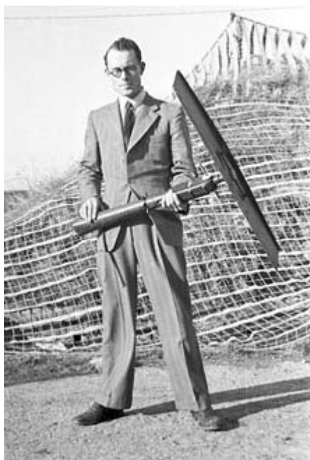
Donald Preist with dipole feed and reflector from the Würzburg radar.
