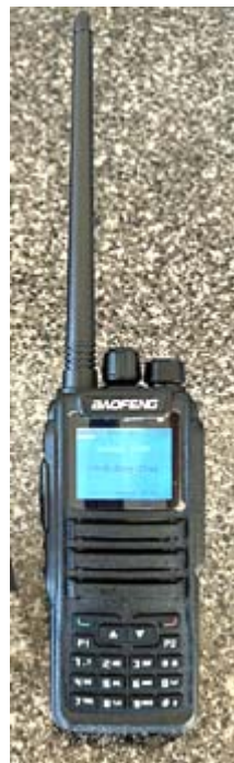
Baofeng DM-1701 dual-band DMR/FM HT. [N2KZ pic.]
