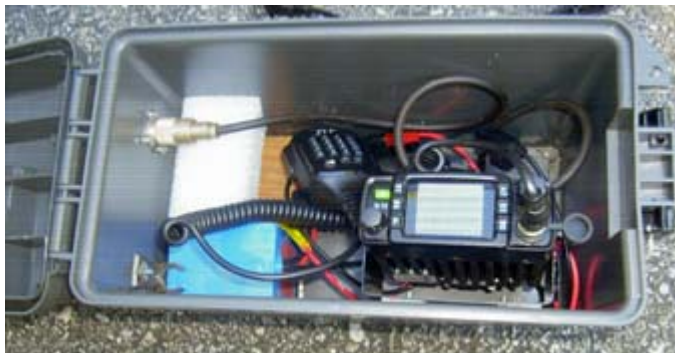
Go-box as described by David KD2EVI in PCARA Update , September 2023. Lower left: 4.5 Ah LiFePO 4 battery with AC charger. Lower right: TYT TH-8600 VHF/UHF transceiver inside the ammo box. [KD2EVI pic.]
