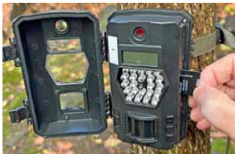
Simmons 10 megapixel Trail Camera with cover open to insert an SD card. [AD2CT pics]
