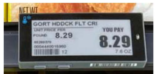
*Shelf label for use inside a freezer case has blue mark, buttons and LED (right).*
