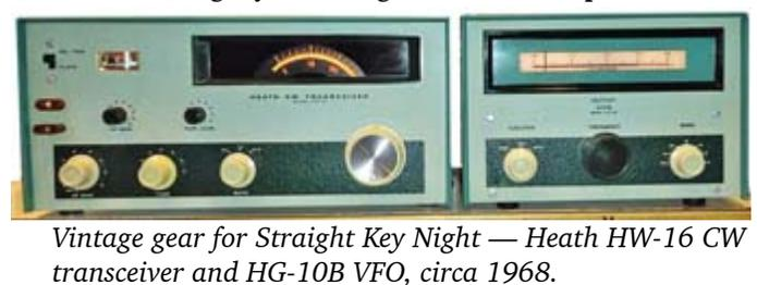
Vintage gear for Straight Key Night — Heath HW-16 CW transceiver and HG-10B VFO, circa 1968.
