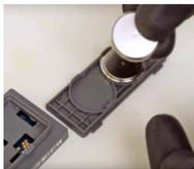
*Changing the two CR2450, 3 volt LiMnO<sub>2</sub> coin cells at the back of a mid-size label. [Solum]*
