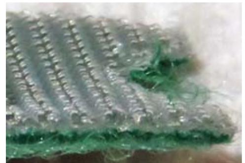
Close-up of last 1/4" of a green Velcro cable tie with molded hooks on top, loops below.
