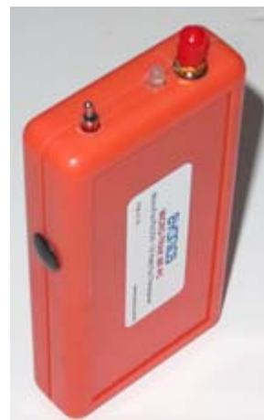
Byonics MicroFox PicCon transceiver in its orange plastic case.
