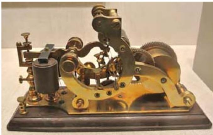
*Telegraph register, 1850. Electromagnets at left attract an iron bar attached to a brass arm, scribing the paper roll.*
