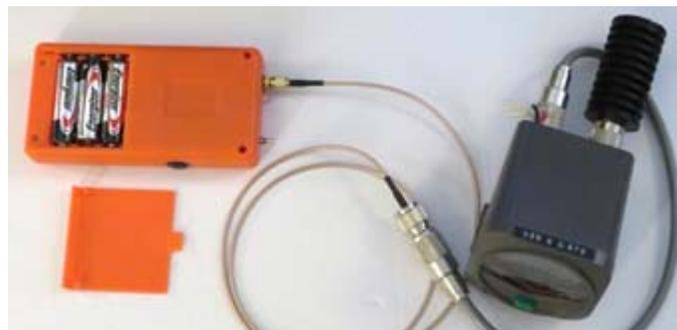
MicroFox test set up using SMA to SO-239 adapter cable, Daiwa power meter and dummy load.
