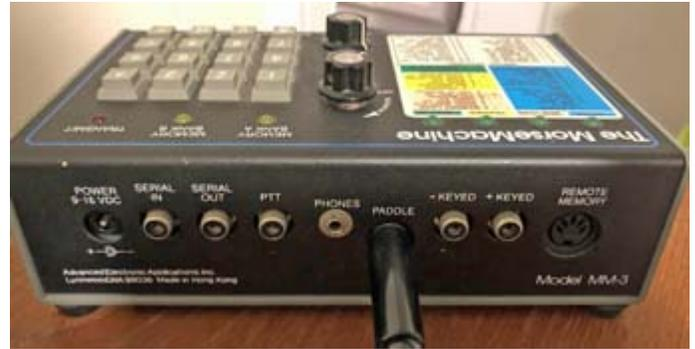
Rear of the MM-3 Morse Machine has connections for power, serial port, phones, straight key or paddle and positive or negative keying for the transmitter.
