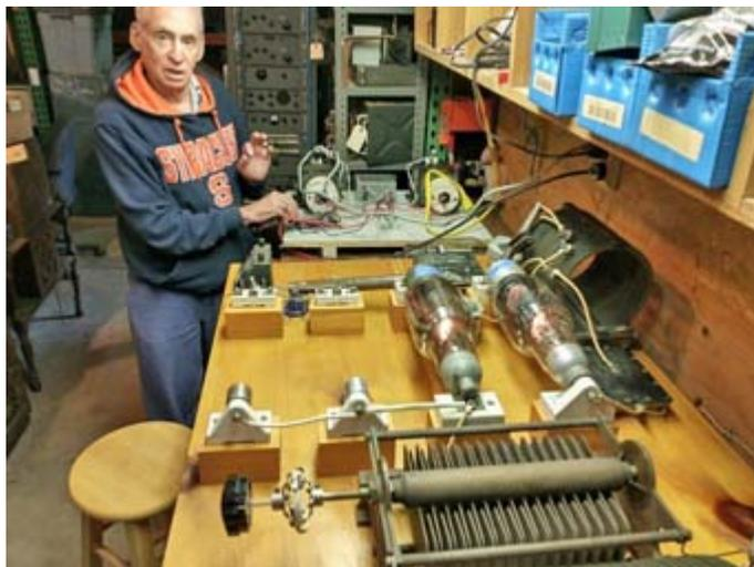
Joel W3ZT tests the 1BCG replica transmitter constructed by volunteers of the Antique Wireless Association. Open layout uses a 204A tube as oscillator and another as PA.
