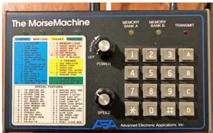
AEA's MM-3 Morse Machine is a Morse trainer, memory keyer and CW beacon. The code proficiency trainer generates random groups with increasing speed. There is also a QSO simulator and contest simulator. The keyer can be set from 2 to 99 wpm with 20 message memories. [W2VJ pics.]
