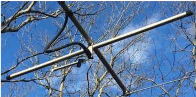
Close-up of the Yagi antenna's driven element. [N2KZ pics.]
