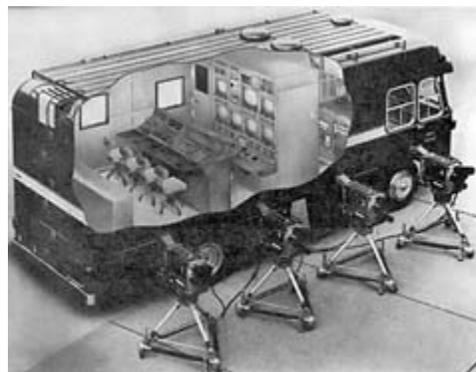
*Pye Mobile Control Room type 844013, with four Mk 6 cameras, cutaway view.*
