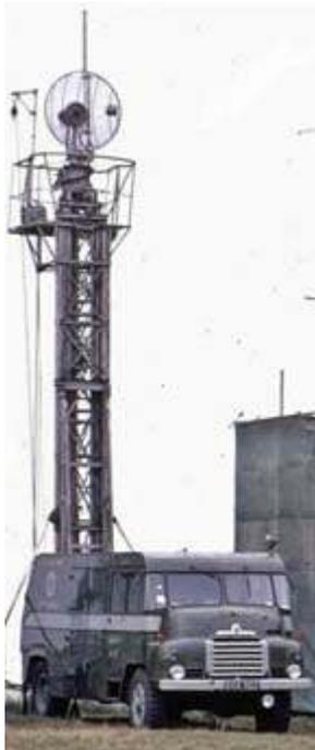
*Eagle Tower raised to vertical position, with microwave dish on top.*
