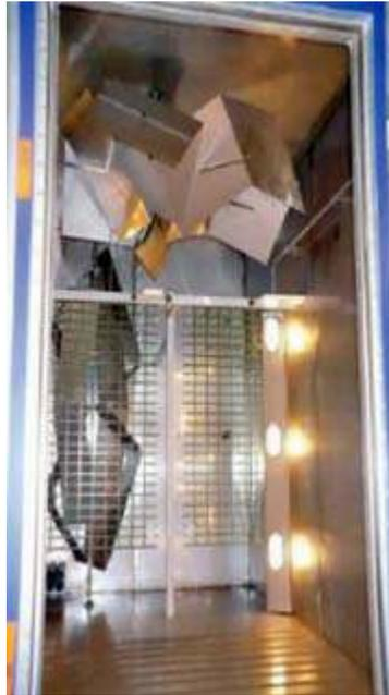
*Empty RF exposure chamber showing horizontal and vertical paddle stirrers to move standing waves around. [Pic credit NTP]*
