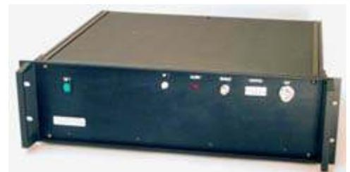
900 MHz 400W custom amplifier by LS Elektronik AB.
