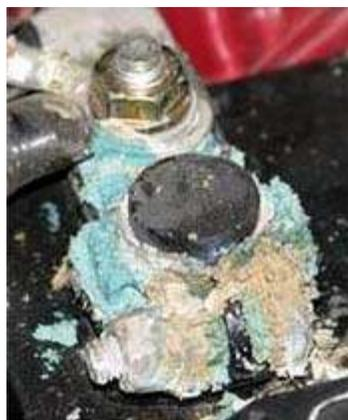
*Corroded copper terminal on a lead-acid battery.*
