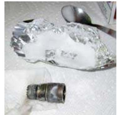
*Cleaning a coaxial adapter with sodium bicarbonate paste.*
