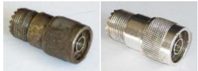
*Before and after pictures of a tarnished coaxial adapter (N-type to SO-239), following treatment with a 3:1 paste of baking soda and water.*
