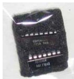
*Static-sensitive components should be placed in conductive foam prior to bagging.*
