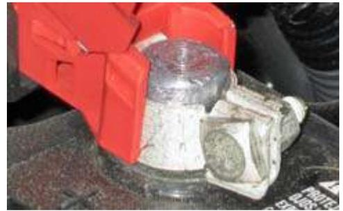
*Normal appearance of a lead-acid battery terminal under its protective plastic cover.*
