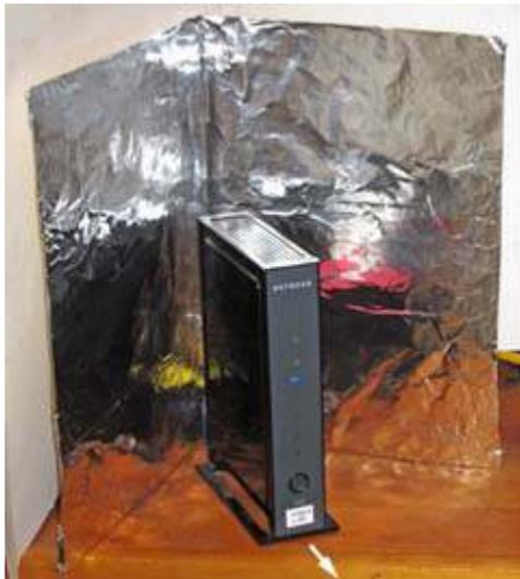
*Corner reflector made from aluminum foil is positioned behind a wireless router or wireless access point to increase range in the direction shown (white arrow).*
