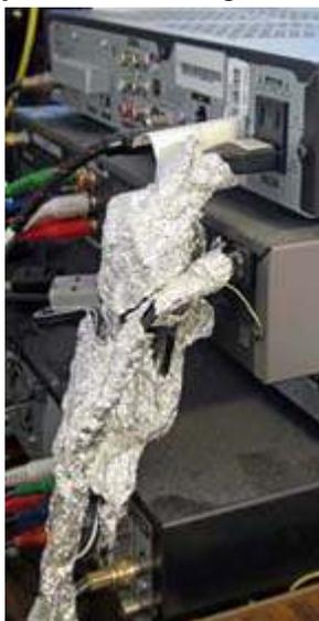
*Use of aluminum foil for additional shielding of audio/video cables.*
