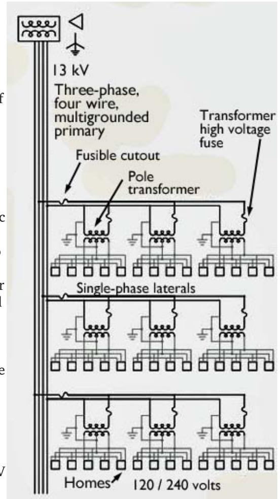
Primary and secondary power distribution. 13 kV three-phase primary with neutral/ground return passes down main road. Each side street is connected to one phase of the 13 kV primary. Along the street, pole-mounted transformers have their primary windings connected between the 13kV line and ground. The secondary winding of each transformer provides 120–0–120V for drop connection to 3–15 homes. [Adapted from electrical-engineering-portal.]
