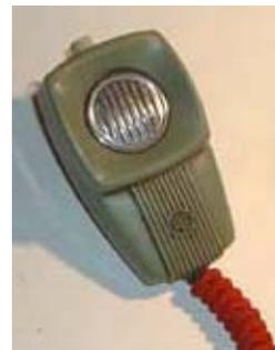
*Pye radiotelephone microphone with press-to-talk button on top.*
