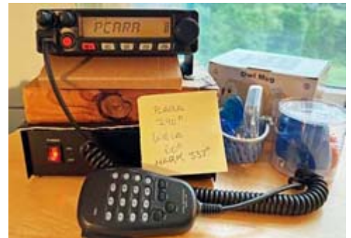
For best coverage from home in a hilly area, use a mobile transceiver with a 12 volt power supply and a good, external antenna. [N2KZ pic.]
