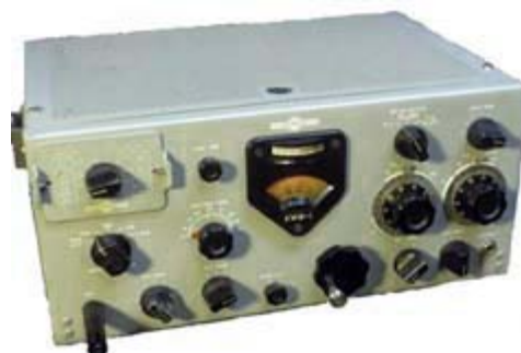
Collins Radio's pioneering KWM-1 transceiver from 1957 covered three HF bands (14 - 30 MHz) with 100 watts PEP out.
