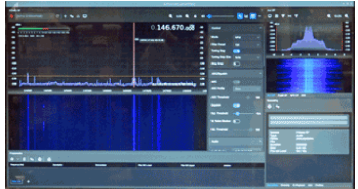
Screen shot of SDRConnect software displaying two meter band during the Old Goats Net. Auxiliary display top right shows spectrum of signal on 146.670 MHz.
