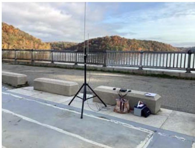
David K2WPM's station at the southeast end of Croton Dam with Baofeng HT, Yaesu FTM-3200D 2 meter transceiver, LiFePO 4 battery, solar back up and VHF-UHF antenna on Pyle tripod. “Ready for anything!” [K2WPM pic.]
