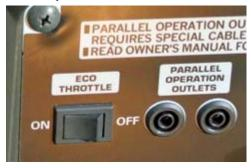
Honda Eco Throttle switch lowers engine RPM when there is a light electrical load.
