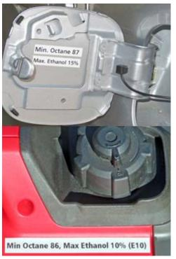
Filler cap labels for vehicle and generator.
