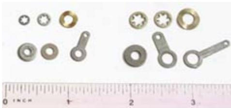
6BA (left) and 4BA (right) lockwashers, washers and solder tags (lugs).
