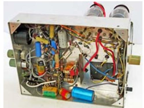
*View underneath the completed modulator project, based on an aluminum chassis.*
