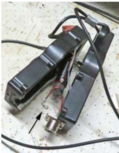
One of the balun input wires was connected to a solder lug (arrowed) no longer connected.
