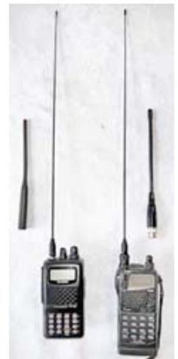
Replace the 'stock' antenna with an extended whip. [N2KZ pic.]
