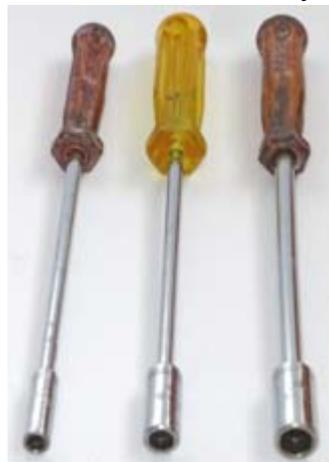
6BA, 4BA & 2BA Spiralux nutdrivers from the UK. Two cellulose acetate/butyrate handles have deteriorated. [PCUD June 2011 p 6.]
