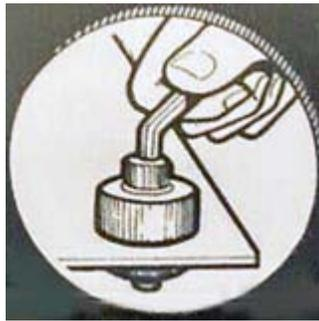
*Q-Max punch can cut a hole in sheet metal up to 16 gauge mild steel. [Q-Max Electronics U.K.]*
