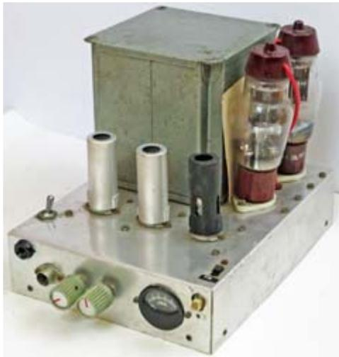
*Example from the early 1970s of an aluminum chassis punched for five vacuum tubes and a panel meter. This was an AM/FM modulator with tube line-up 12AX7 – 12AX7 – 12AT7 driving a pair of 807s for 30 watts audio output.*
