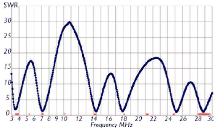
Graph from Microsoft Excel shows SWR plotted against frequency for off-center fed dipole, overall length 136 ft.
