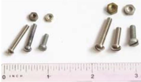
6BA size (left) and 4BA (right) bolts and nuts as used in British electronic equipment in the 1960s. They are mostly obsolete, replaced by ISO metric sizes today.
