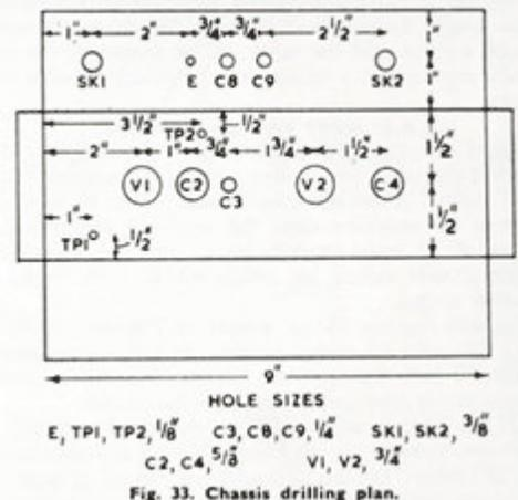
Chassis layout showing holes for vacuum tubes V1, V2 and other components C2, C4. (*RSGB Handbook*).
