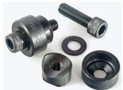
Q-Max chassis punch (left) and its four components: punch, die, washer, screw.
