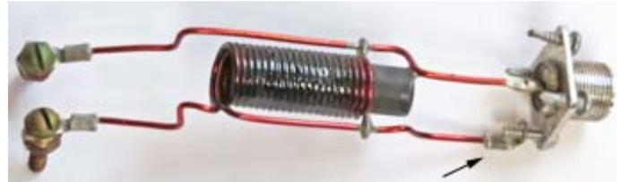
4:1 balun removed from its plastic enclosure. Enameled wire around ferrite rod core is discolored and the core has shifted. Solder lug with missing nut arrowed.
