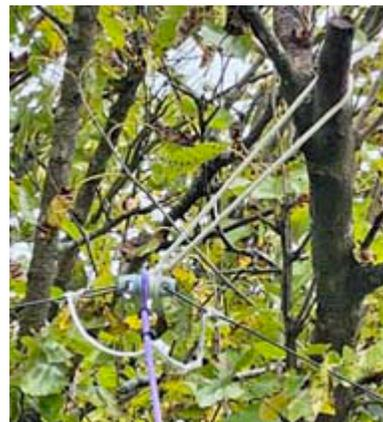
Dipole center insulator supported by rope loop. [N2KZ pics.]
