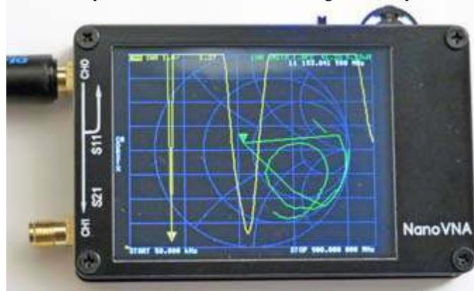
Yellow trace shows SWR of Diamond SRH519 dual-band SMA antenna. Marker 1 at 153 MHz, next dip at 432 MHz.
