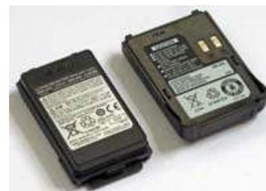
Lithium-Ion HT batteries (7.2V) by Yaesu and Kenwood.
