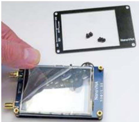
The protective film over the touch-screen can be peeled off after removing the bezel.
