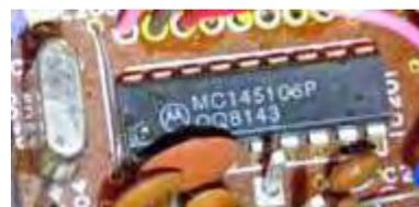
*Motorola MC145106 frequency synthesizer IC in Icom ICB-1050.*
