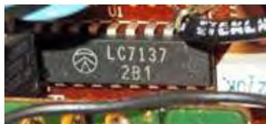
*Sanyo LC7137 PLL frequency synthesizer integrated circuit in a Rotel CB radio..*
