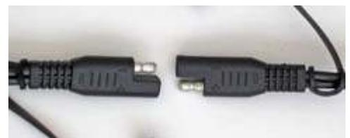
SAE 'bullet' connectors on the charger and battery cables.
