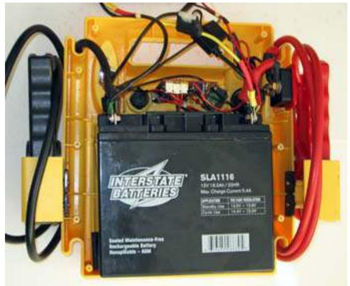
Superex portable power supply with the new SLA1116 AGM battery. Cables are already in place for the Battery Tender Jr charger and external Powerpole connection.
