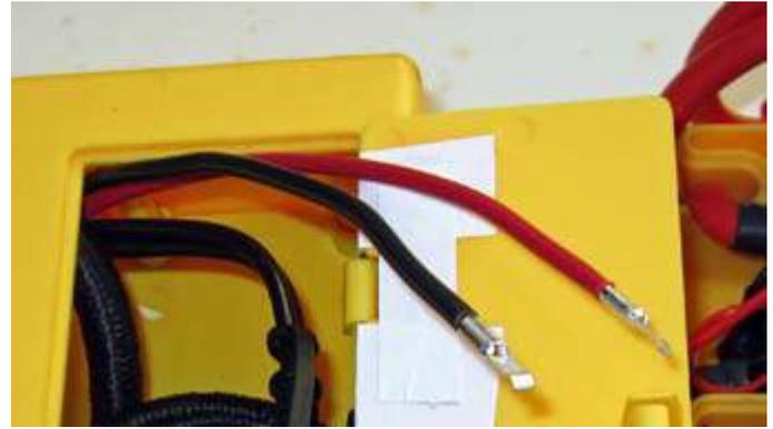
12 AWG cable with Powerpole contacts threaded into position in the storage compartment *before* insertion of silver-plated contacts into the Powerpole plastic housings.
