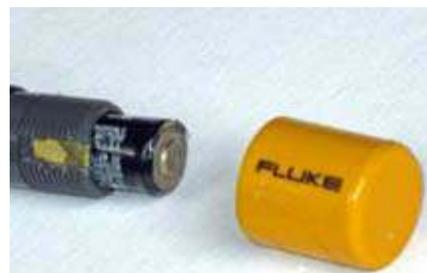
Fluke VoltAlert AC voltage detector after cleaning the bad battery.
