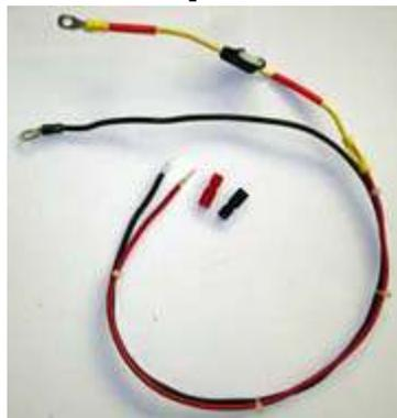
New cable with ring terminals, fuse and Powerpole contacts.
