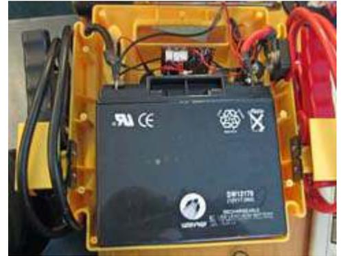
*Removing the back of the yellow plastic case reveals the original SW12170 battery.*
