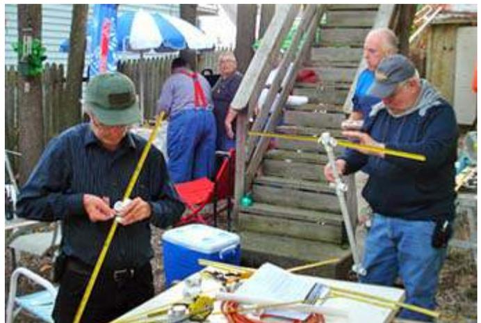
*Tape measure Yagi construction by CARA. [Pic KD2GJJ]*
