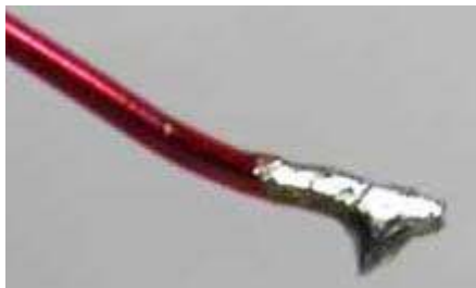
Polyurethane enamel can be removed by heating the wire with a soldering iron.
