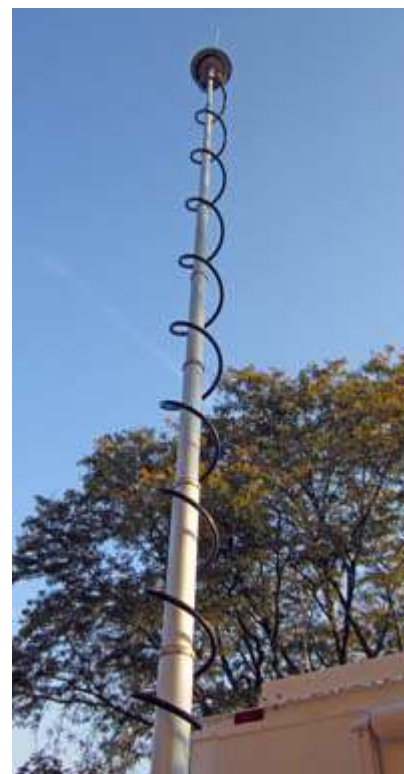
The hydraulic mast on the back of the RACES truck extended to its full height of 42 feet.
