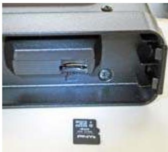
MicroSD memory card ready to be inserted into the body of the radio. The notch should be to the left, not as shown.
