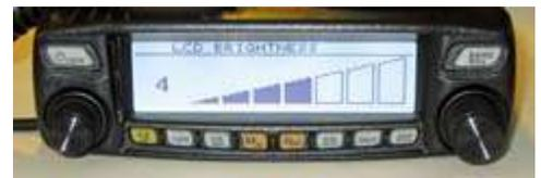
Brightness of the LCD backlight can be adjusted using: DISP→1 DISPLAY→2 LCD BRIGHTNESS, then rotate the control knob.
