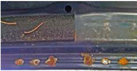
Rust spots under the lid of Karl's trunk show where the Diamond NR22L antenna was originally mounted.
