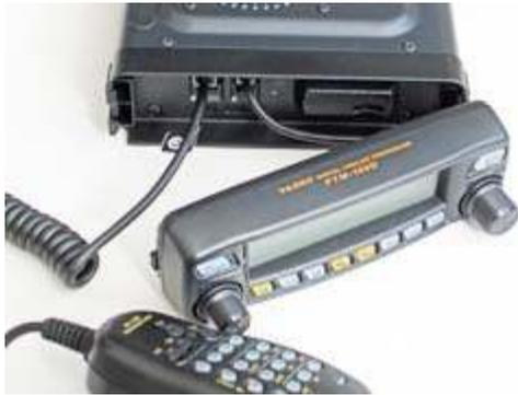
The control head must be detached in order to connect the MH-48 microphone.
