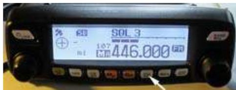
*Squelch adjustment using the 'SQL/VOICE' button on the FTM-100D front panel.*
