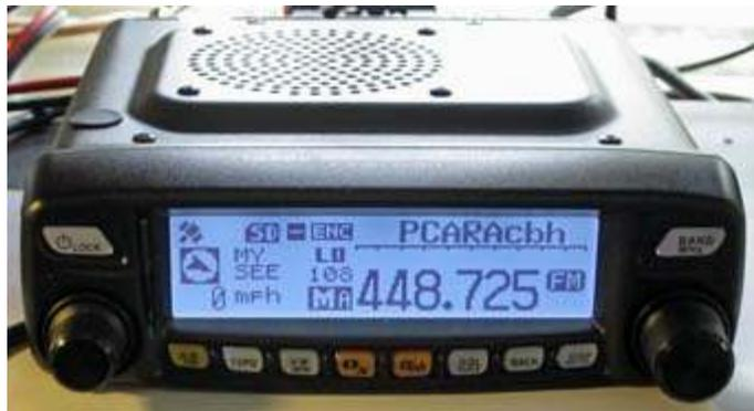
*Example of a stored memory channel with (small) name displayed on the upper line of the LCD display.*
