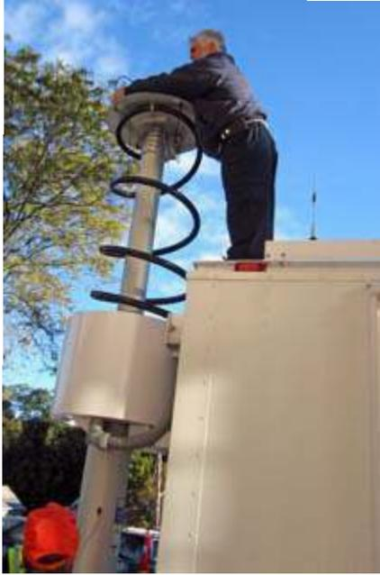
*Bob, N2DVQ changes antennas on the telescopic mast mounted at the back of the RACES vehicle..*
