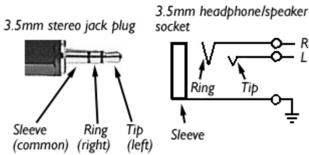
Right-channel output from a 3.5mm stereo socket to a stereo jack plug would be shorted out by a mono plug.
