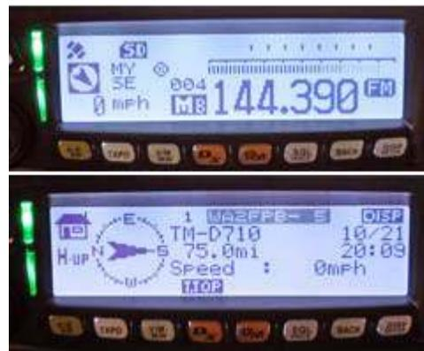
*With the radio tuned to the appropriate frequency and the APRS modem turned on, incoming data are displayed.*
