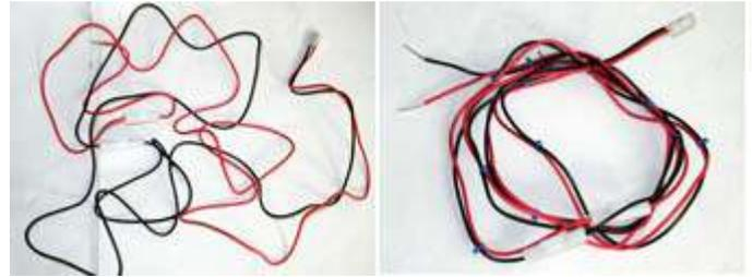
The DC power cable had its red and black wires separated (left). This was fixed with cable ties every 8 inches.
