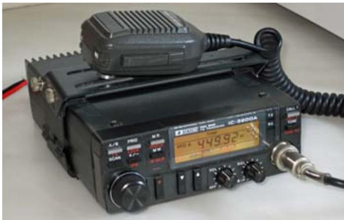
*Icom IC-3200A dual-band mobile FM transceiver for 144 and 440 MHz is still working.*
