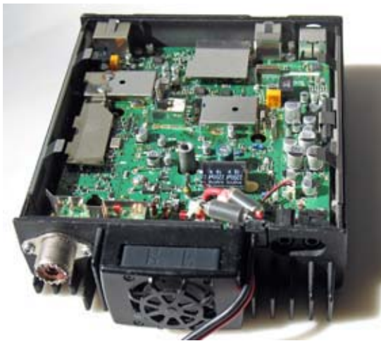
View inside the main unit of the IC-2800H with the cover off. The cooling fan draws in air from the rear.
