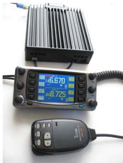
The Icom IC-2800H dual band FM transceiver has a diecast main unit, a separate control head with LCD color screen and an HM-98 hand microphone.
