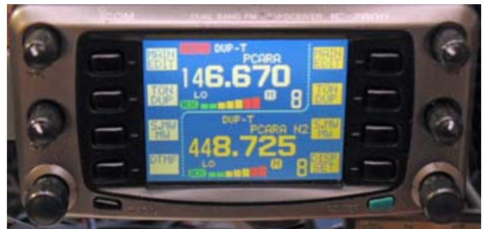
Close-up of the IC-2800H remote control head. Both frequencies were in use at the time of this photo!
