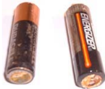
When good batteries go bad... heavily corroded AA cells.
