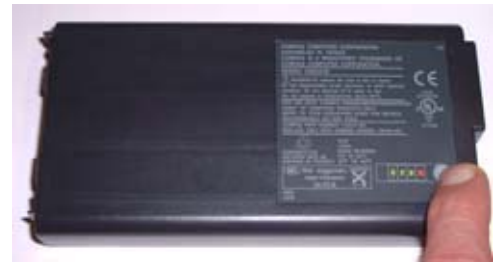
Compaq lithium ion notebook battery has its own circuitry to indicate state of charge and regulate charging current.
