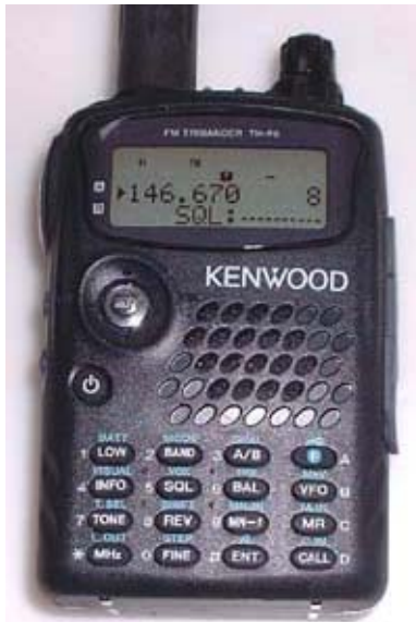
You can drain the battery of a handi-talkie like this Kenwood TH-F6 by opening the squelch.
