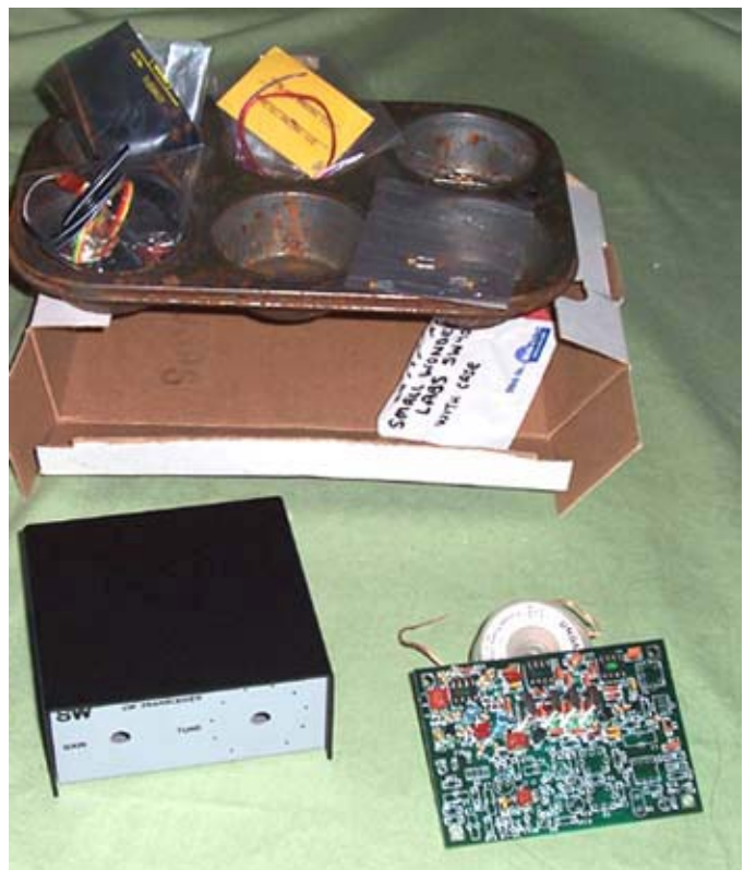
Small Wonder Labs SW+ 40 meter CW transceiver kit, complete with currently-discontinued enclosure kit.
