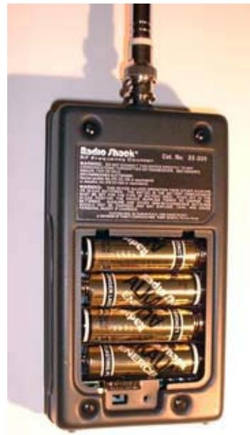
*Don't forget to check batteries in your test equipment. Picture shows a Radio Shack LCD RF frequency counter.*
