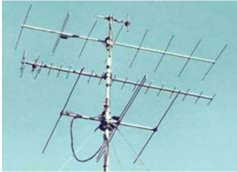
VHF/UHF antennas at home. From top to bottom, 432 MHz vertical, 144 MHz 8-element Yagi, 432 MHz Parabeam and U.K. 70 MHz band 3-element Yagi.
