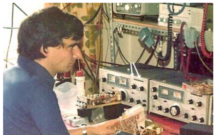
Yaesu/Sommerkamp separates — FL-dx500 transmitter and FR-dx500 receiver from 1960s-70s. Transmitter Plate (Tune) and Load controls are arrowed.
