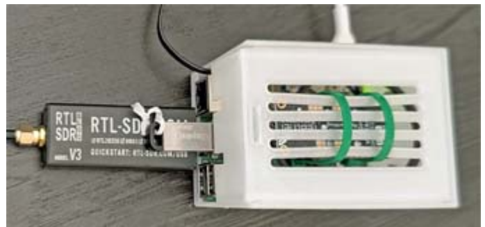
RTL-SDR dongle plugged into USB port of a Raspberry Pi 5 single board computer. [KE2JEN pic.]
