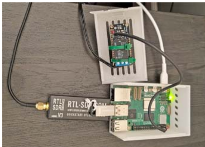
Raspberry Pi with case open to show the Power Relay Featherwing. [KE2JEN pic.]
