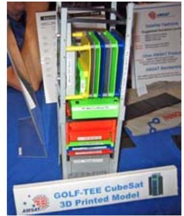
3D-printed mock-up of CubeSat linear satellite.
