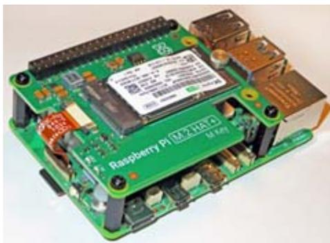
*512 GB solid state drive inserted into the Raspberry Pi M.2 HAT+.*
