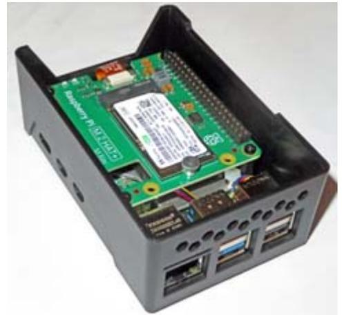
*HighPi Pro 5S plastic case with Raspberry Pi 5 and solid state drive mounted inside. The ventilated case lid, which clips on top, is not shown.*
