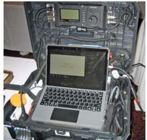
Lab599 Discovery TX-500 10W portable radio with Digirig digital modes interface set-up in portable case by Smitty KC1IKA.
