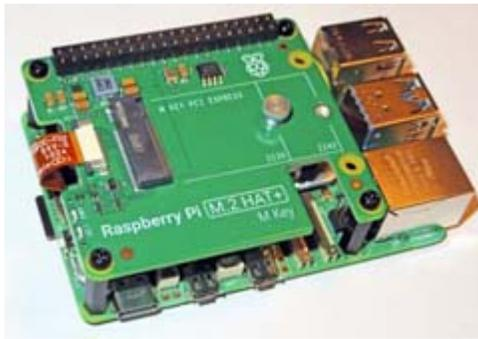
*Raspberry Pi M.2 HAT+ installed on top of the Raspberry Pi 5*
