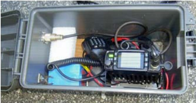
Go-box described by David KD2EVI in PCARA Update, September 2023. Lower left: 4.5 Ah LiFePO<sub>4</sub> battery with AC charger. Lower right: TYT TH-8600 VHF/UHF transceiver inside the ammo box. [KD2EVI pic.]
