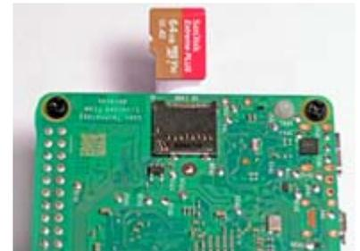
*Inserting a 64GB microSD card into the Raspberry Pi 5.*
