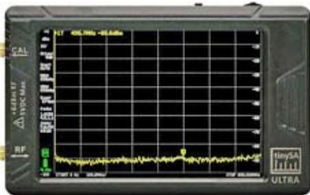
4-inch screen tinySA-Ultra spectrum analyzer. [<https://www.tinysa.org/wiki/>]
