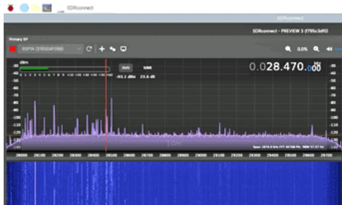
Partial screenshot of SDRplay's SDRconnect software running on the Raspberry Pi 5. Spectrum shows SSB signals in the 10 meter band received on RSP1A during IARU Region 1 SSB Field Day, September 8, 2024.
