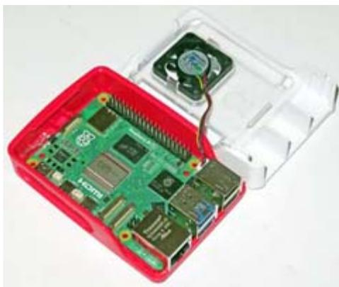
*Raspberry Pi 5 board mounted in the official case. White frame contains the case fan, which is wired to the board.*
