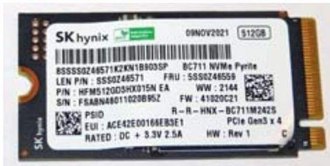
*SK hynix 512 GB solid state drive in 2242 size. "M.2 M key" specifies an M.2 edge connector with 5 contacts alongside the notch.*
