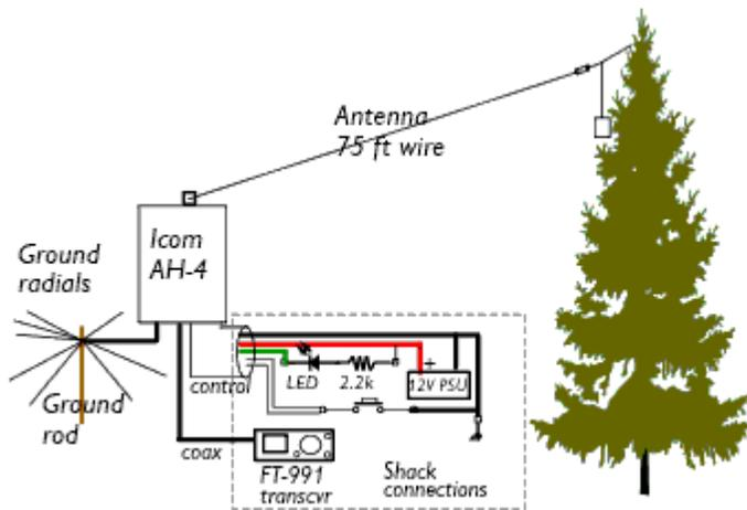
Connection of an end-fed long-wire antenna and ground system to an Icom AH-4 antenna tuner as described by Bob N2CBH in PCARA Update for October 2018. [N2CBH diag.]
