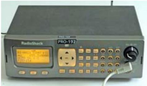
*Radio Shack PRO-197 digital trunking scanner receiving P25 Phase 1.*
