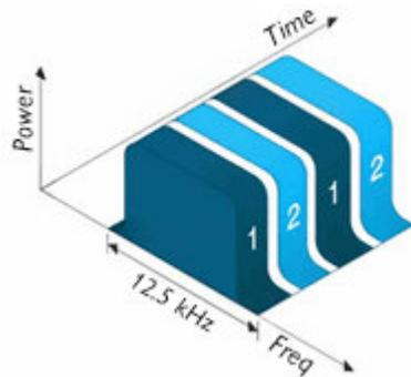
*P25 Phase 2 employs TDMA, with two time slots, each slot carrying a different voice channel.*
