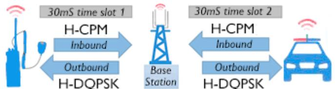
*P25 Phase 2 employs two-slot TDMA within a 12.5 kHz voice channel, with different modulation schemes inbound and outbound.*
