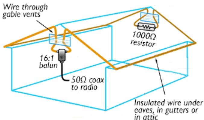
Broadband Butterfly Terminated Dipole Antenna covers 1.8 - 54 MHz with SWR <2:1. Total wire can be any length to fit around house perimeter. 1000Ω terminating resistor should have same power rating as transmitter output. [After Bonnie Crystal KQ6XA.]
