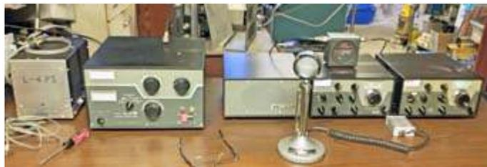
Bob's Drake inventory, L to R: L-4PS Power Supply, L-4B amplifier; MS-4 speaker with AC-4 power supply, T-4XC transmitter and R-4C receiver. [N2CBH pics.]
