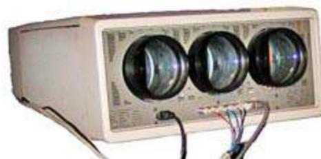
NEC DP-1200 video projector had three cathode ray tubes and three lenses for red-green-blue output at VGA resolution.
