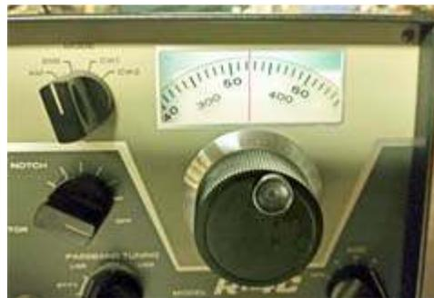
Drake main tuning control and tuning dial. Main tuning knob can be held stationary while adjusting the skirt.
