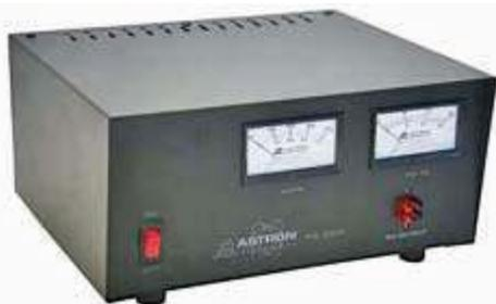
Astron RS-35M-AP linear power supply is rated at 13.8V DC, 35A peak output, 120V AC input, with front panel meters and Anderson Powerpole Connectors.
