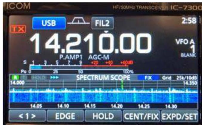
Spectrum-scope display of IC-7300 shows switch mode power supply harmonics every ~33 kHz. [W2VJ pic.]
