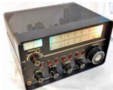
Drake 2B receiver covered 80 - 10 meter bands, SSB, CW and AM.
