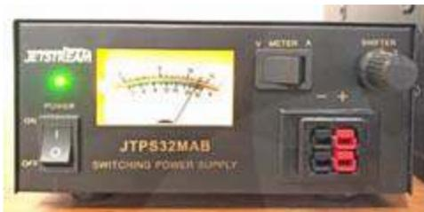
Jetstream JTPS32MAB is rated 30A peak, 25A continuous, with meter, 'Shifter' knob and Powerpole connectors on the front panel. [W2VJ pic.]
