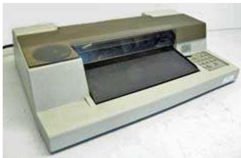
HP 7475A plotter with 6-pen carousel and moving paper mechanism.
