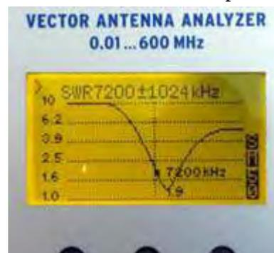
Screen plot of SWR for multiband sloper antenna on 7 MHz.
