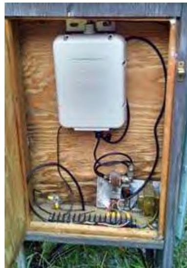
Icom AH-4 tuner mounted in the wooden shelter. [N2CBH pic.]
