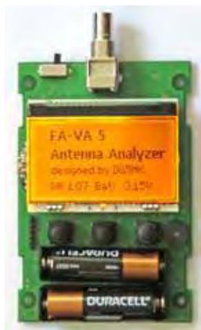
Functional test before final assembly shows instrument working.
