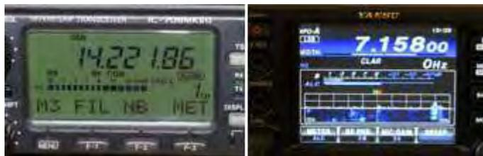
Icom IC-706MkIIG monochrome display is on the left, FT-991A color touch display on the right.
