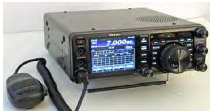
*Fresh out of the box, the FT-991A powers up on 7.0 MHz, VFO-A and lower sideband.*
