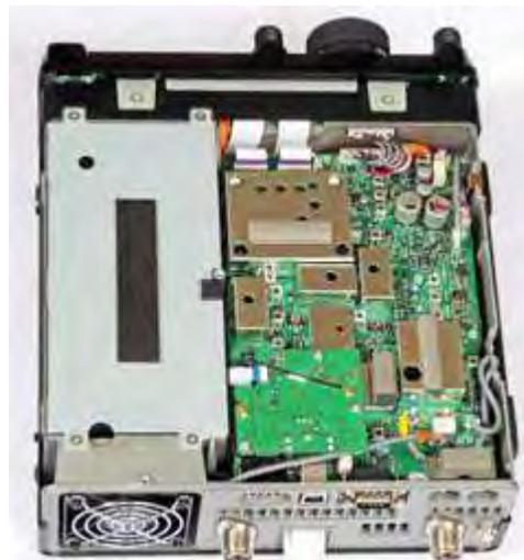
With the FT-991A bottom cover removed, automatic antenna tuner is located behind the rear cooling fan, under the shield case cover.
