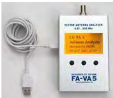
FA-VA5 Antenna Analyzer with USB A-to-mini-B cable.
