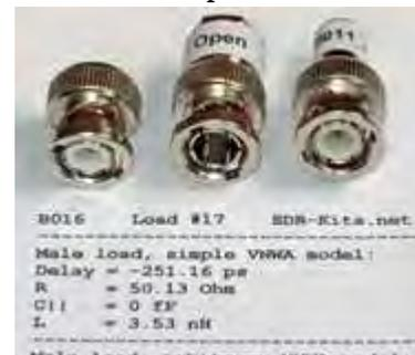
SDR-Kits' Short / Open / Load male BNC calibration kit with measured data sheet.
