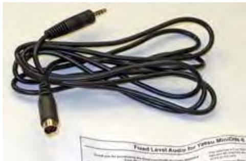
West Mountain Radio fixed level audio cable for Yaesu Mini-DIN 6-pin connector.
