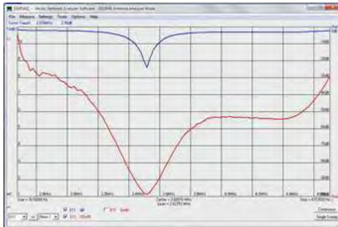
Screen shot of VNWA software as it plots multiband sloper’s VSWR in red (vertical scale 1-10) and Return Loss in blue (vertical scale 0 to -100 dB). Horizontal frequency scale covers 2.8 - 4.6 MHz, centered on 3.6 MHz.
