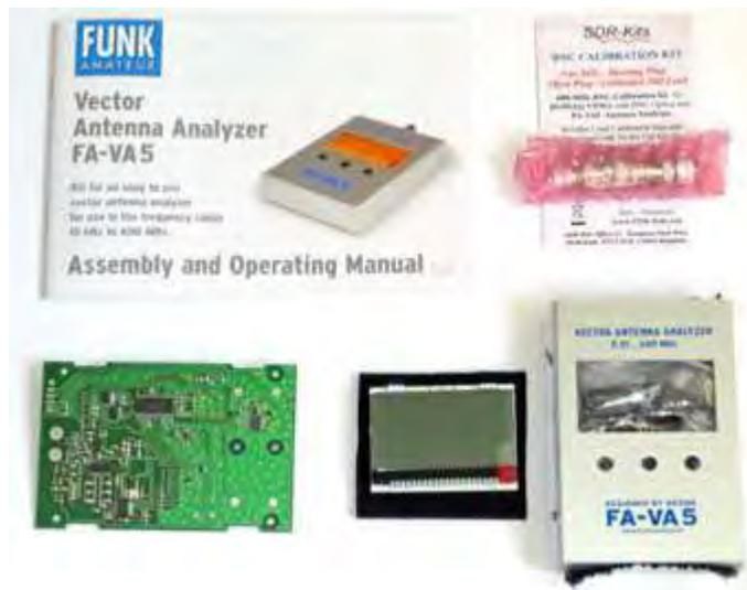
FA-VA5 Analyzer Kit includes a circuit board with SMD parts, display panel, aluminum case and other components.
