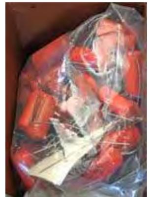
Sprague Orange Drop® capacitors with Mylar dielectric and epoxy coat.
