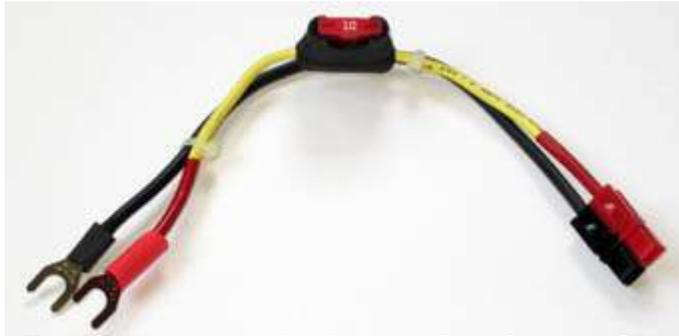
Home-brew power supply adapter with spade terminals at one end, 10 amp inline ATC fuse in the middle and Anderson Powerpoles at the other end.
