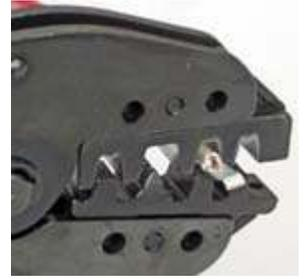
*Ensure contact is level with hook pointing down.*
