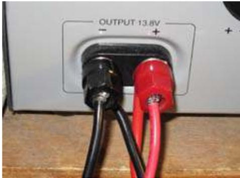
*Original binding post connections on a RadioShack linear power supply.*
