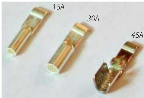
*Contacts for use with Powerpole PP15-45 series plastic housings. Left: silver-plated closed barrel contact for 16 to 20 AWG wire. Center: silver-plated contact for 12 to 16 AWG wire. Right: tin-plated open barrel contact for 10 to 14 AWG wire.*
