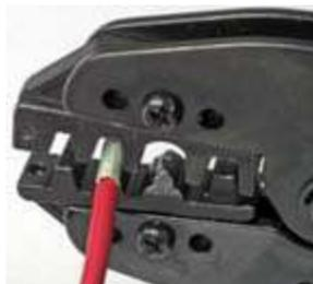
*Place wire + barrel into crimping tool, seam up.*
