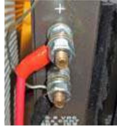
The next power supply to be upgraded had binding posts with color-coded caps that screw down onto threaded connectors. Ring terminals would not be suitable for this type of adapter as the power supply screw-caps are **captive**. I made up my own adapter cable with **spade lugs** that would slide securely under the binding posts.
