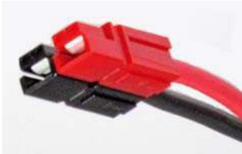
*ARES/RACES standard for physical arrangement of Powerpole housings can be remembered as tongue top, red right.*
