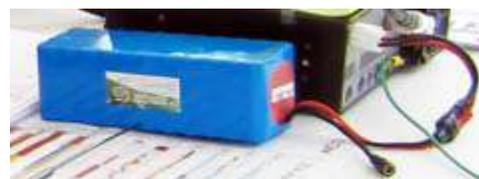
Close-up of the Bioenno LiFePO<sub>4</sub> battery
