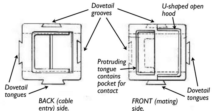
Drawing of dovetail tongues and grooves plus mating parts of a Powerpole housing, from U.S. Patent 3,259,870.
