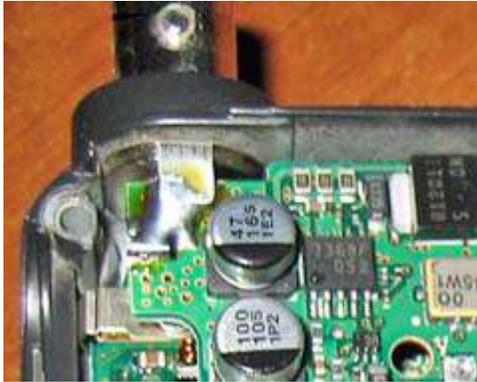
Close-up of Icom IC-T7H BNC antenna socket with ground tab soldered to the "2F unit" circuit board, top left. Tip of the BNC socket is connected to the "1F unit" board mounted below.
