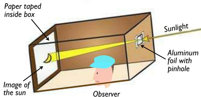
Pinhole projector box. Bottom of the box is left open.
