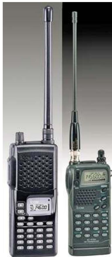
*Original Icom IC-T2H single band transceiver (left) and its dual-band replacement IC-T7H (right)*
