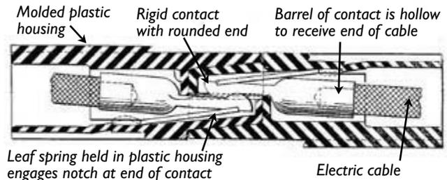
Drawing of Anderson Powerpole genderless connectors, adapted from U.S. Patent 3,259,870
