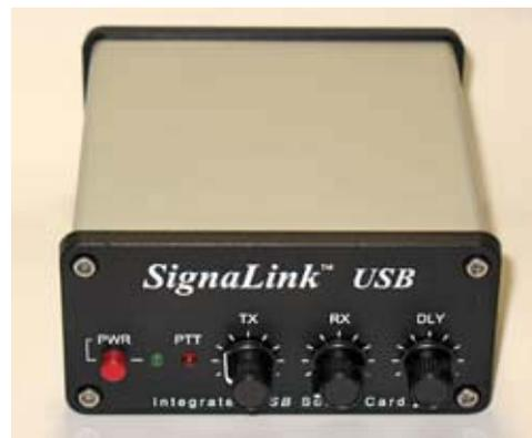
*Tigertronics' Signalink USB has an integrated USB sound card.*
