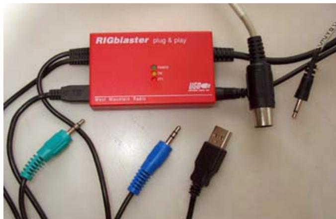
*The RIGblaster “plug & play” sound card interface has lots of connectors for (L-to R) PC output audio, PC input audio, USB, transceiver data and transceiver control.*
