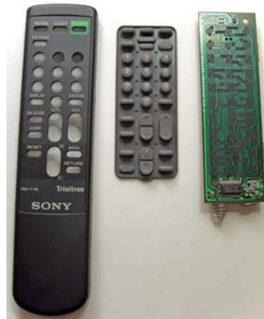
Inside a Sony remote control. Left to right, plastic case, rubber keyboard and printed circuit board.
