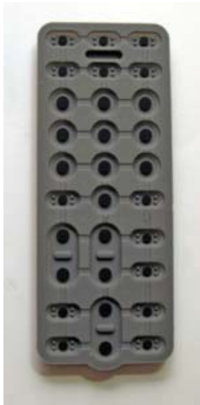
Underside of the rubber pad from the Sony remote control on p 3. Black circles are conducting rubber.
