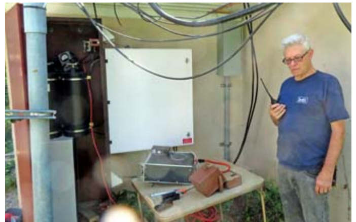
Bob N2CBH checks operation of the 2 meter repeater using RF test equipment on the table.
