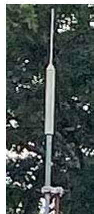
Sleeve dipole antenna in FDR State Park.
