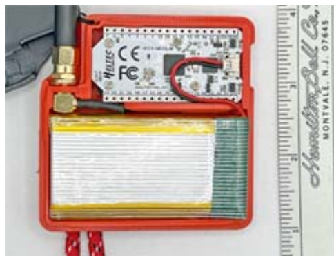
Inside the node, showing the Heltec V3 board (reverse side), 3000 mAh battery, and antenna. [AD2CT pics.]
