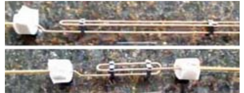
VHF (top) and UHF folded sections from a Comet GP-9. Black plastic clips hold folded sections. PU foam keeps wires centered.
