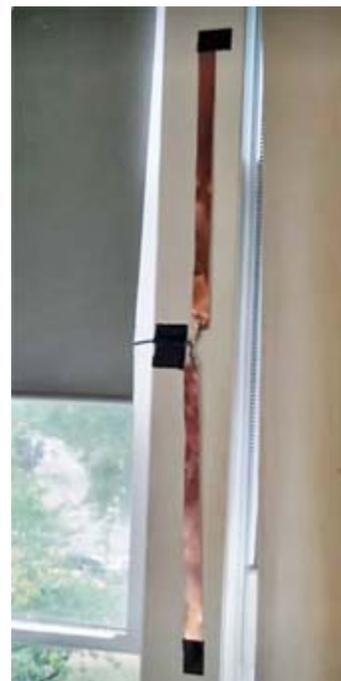
*Copper foil dipole for 2 meters taped to window frame. [K2DMV video.]*
