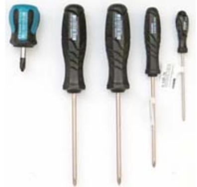
JIS-specification screwdrivers from Vessel and Hozan.
