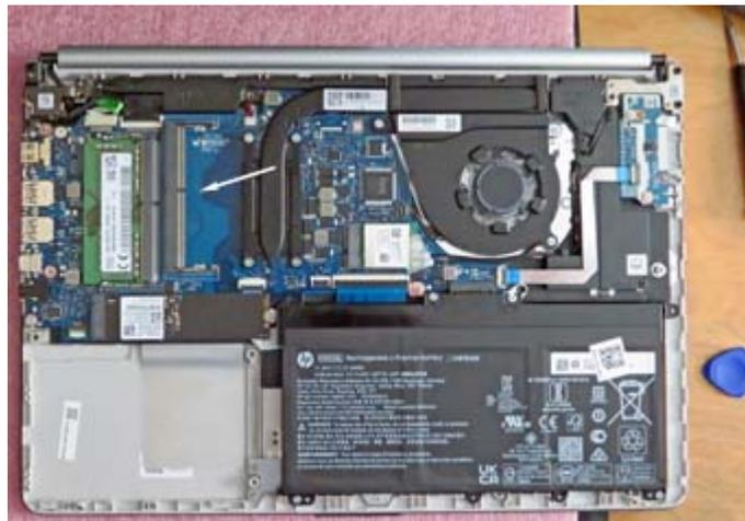
Bargain basement HP notebook with bottom cover removed and slot for additional memory arrowed. Spudger at right.
