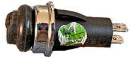
*Faulty press-button switch removed from Weber grill [N2KZ pic.].*
