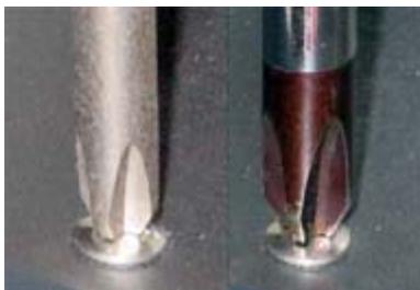
A #2 JIS screwdriver (left) fits precisely into a JIS screw, while a #2 Phillips screwdriver (right) does not fully seat.
