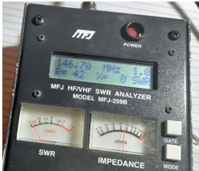
*Al adjusted lengths of the copper foil dipole elements for an SWR of 1.0:1 in the 2 meter band.*
