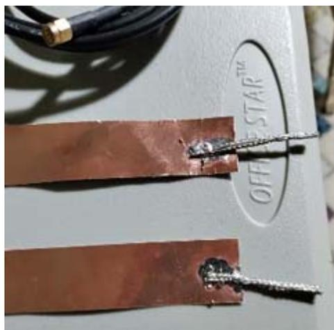
*Al K2DMV was able to solder tinned braid wires to the copper foil tape.*
