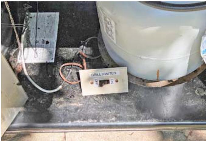
*Karl substituted an old light switch for the faulty press-button igniter on the Weber grill. [N2KZ pic.]*
