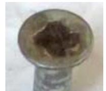
*Damaged recess in Phillips screw.*
