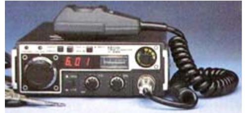
Icom IC-280 2 meter FM transceiver from 1978 was the first model to include a microcontroller. It had three memories and a detachable front-panel unit.
