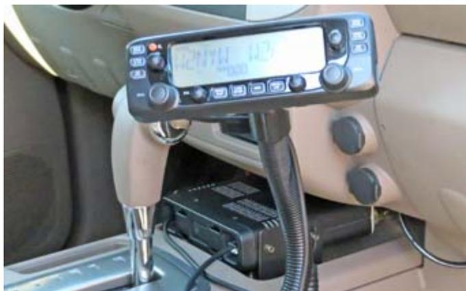
*Body of the IC-2730 transceiver is installed separately from the control head on an Icom MBF-4 mobile mounting bracket, screwed to the shelf on the center-front console.*
