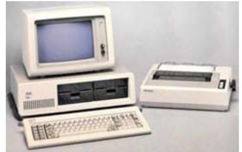
*The original IBM PC of 1981, with twin diskette drives, monochrome display, keyboard and dot matrix printer.*
