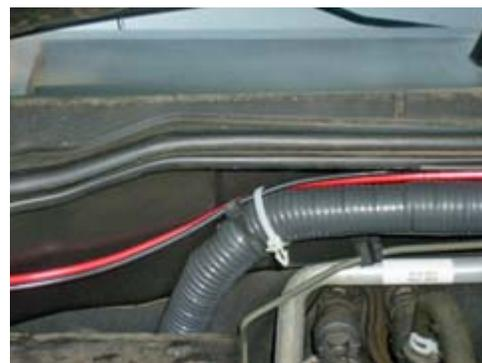
*10 gauge red/black cable fastened to the wire loom that passes from engine compartment through the firewall. [KD2EVI pic.]*
