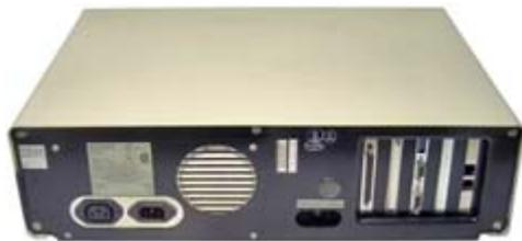
*Rear of the IBM PC's well-shielded metal case with connectors for power out/in, keyboard/cassette and 5 expansion slots.*
