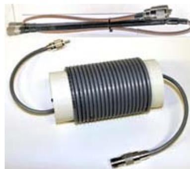
Top: W2DU-style ferrite choke balun. Below: "ugly" coax choke balun wound on plastic pipe.
