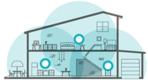
*TP-Link Mesh WiFi units deliver seamless coverage and connect a whole home — in contrast with range extenders that add coverage but create separate networks.*
