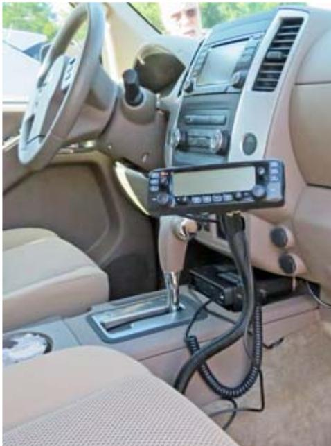
*Icom IC-2730 control head installed on a 'Lido Seat Bolt Mount' inside Frontier cab.*
