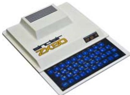
*Sinclair ZX80 microcomputer based on the Zilog Z80 8-bit processor.*
