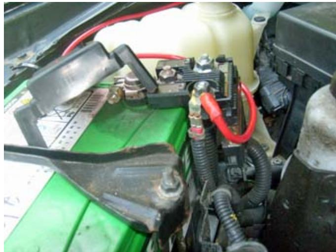
*10 gauge (red) wire is secured to the fusible link assembly on the Nissan's battery positive terminal. [KD2EVI pic.]*
