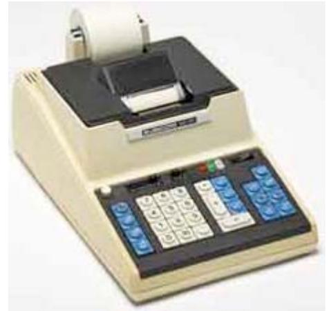
Busicom 141-PF desktop printing calculator from 1971 with one Intel 4004 microprocessor, two 4002 DRAMs, three 4003 shift registers and four 4001 ROMs.
