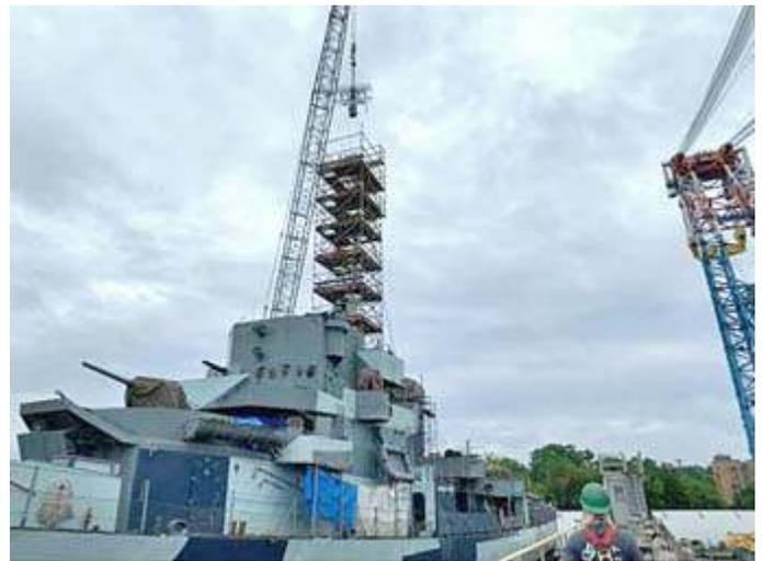
*Restored air search radar antenna is returned to Slater's mast, now surrounded by scaffolding. [Pic credit DEHM].*
