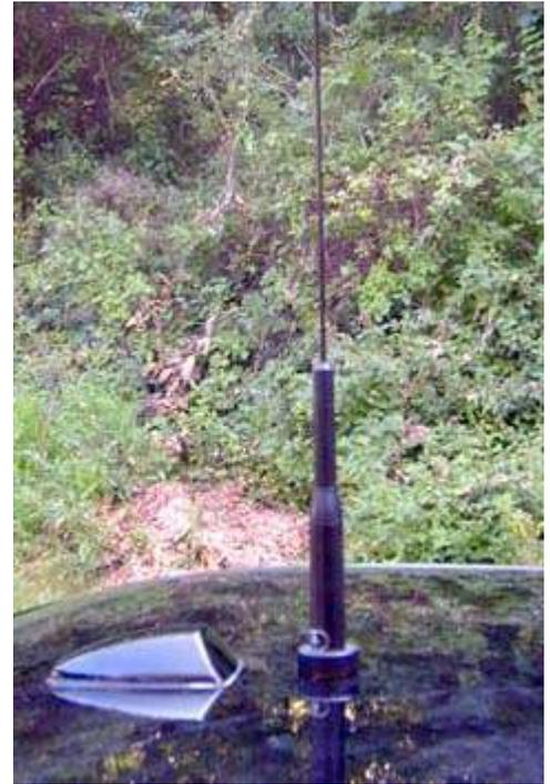
*Comet SBB5 dual-band antenna on the newly-installed NMO-mount. [KD2EVI pic.]*
