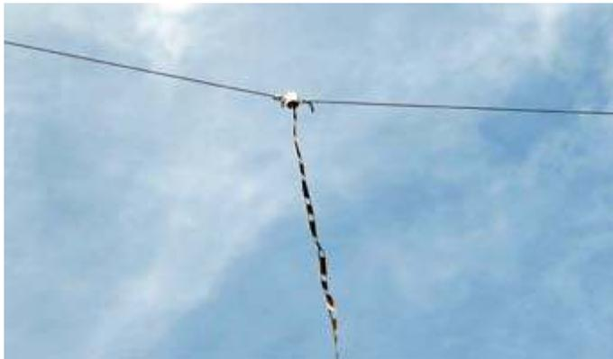
Joe WA2MCR's commercial version of the ZS6BKW antenna.
