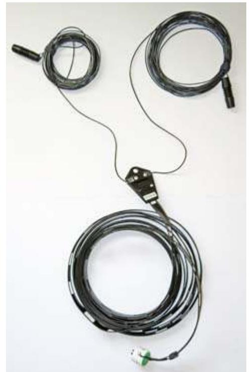
Home-built ZS6BKW antenna using 14 gauge stranded copper wire with black insulation and 450 ohm ladder line.
