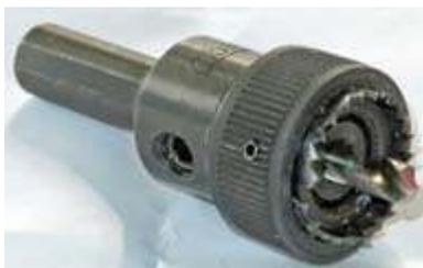
*Cablematic® 3/4" hole saw as used to drill hole for NMO mount.*
