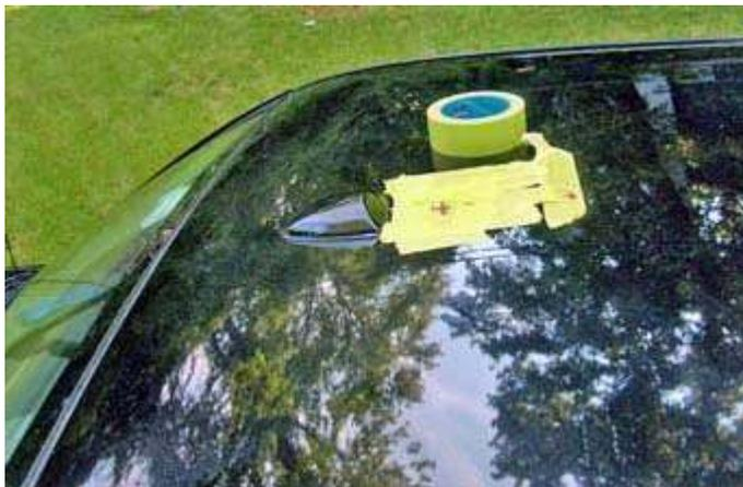
*The position to drill was marked on the pickup's roof using 3M yellow masking tape. [KD2EVI pic.]*
