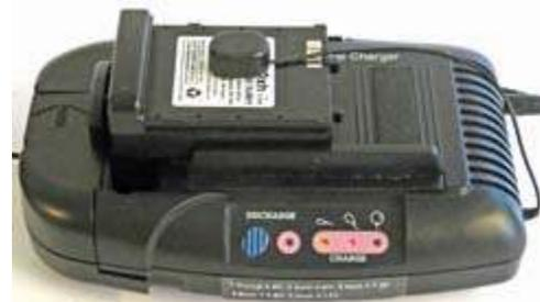
Maha MH-C777 Charger/Conditioner, purchased long ago at a PCARA Bring & Buy sale from Ray W2CH. The Maha unit has a discharge/charge capability designed to bring NiCd and NiMH battery packs back to life. It can discharge a dubious battery pack into a resistive load down to a safe voltage, then recharge the pack while monitoring voltage and temperature to avoid overcharging.
