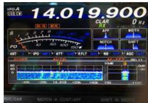
Yaesu FT DX 1200 4.3" TFT color display with S-meter and spectrum scope.
