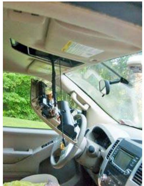
*NMO mount and cable dangles down next to the dome light assembly after being fished across the roof. [KD2EVI pic.]*
