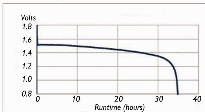
Discharge curve for an AA-size lithium iron disulfide cell, discharged at 100 mA rate to a 0.9 volt cutoff. [Energizer]
