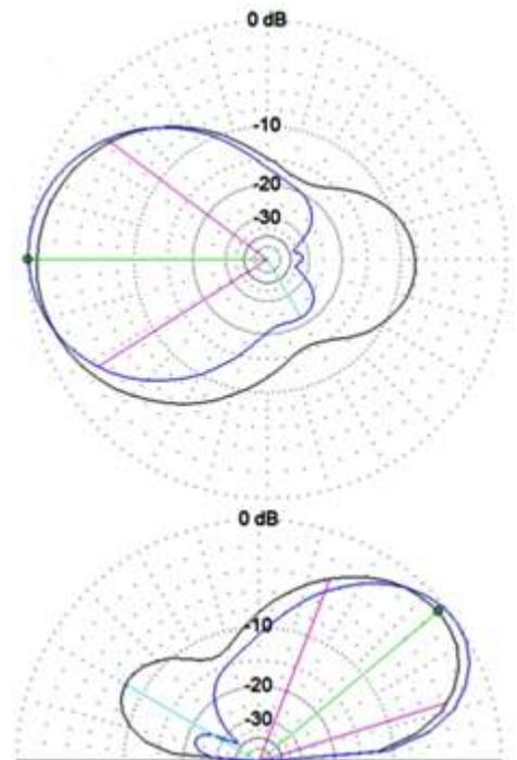
Fig 3. Azimuth (top) and elevation patterns (below) for wire beam antennas at 7.14 MHz as modeled by Jay NE2Q. Black trace is for 2-element beam with 8dBi gain, blue trace is for 3-element beam with 9.2dBi gain (including ground reflections) and improved F/B.
