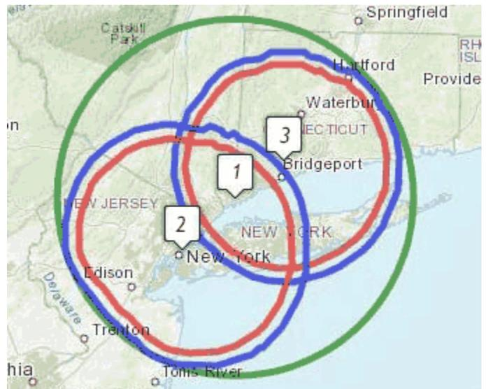
WEDW will reach up to 73 miles — green circle — from Stamford, CT ①, using two separate DTS transmitters, both on RF Channel 21 and located at ② the Empire State Building and ③ Trumbull, CT. [After rabbitears.info]
