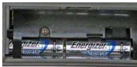
Sony ICF-2010 LW/MW/SW/FM receiver (top) has been fitted with two lithium AA cells in the battery compartment to maintain clock and memory contents.
