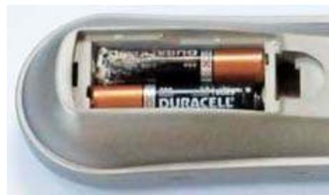
What you **don't** want to see inside a remote control. The AA batteries have discharged and leaked electrolyte.
