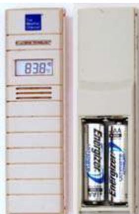
Weather station outdoor TX unit is powered by two lithium AA cells.
