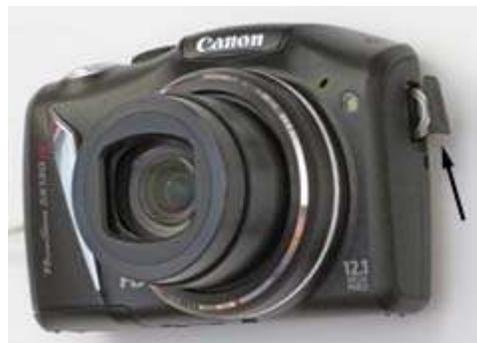
Canon SX-130 camera has a CR1220 coin cell (arrowed) to maintain the date/time.
