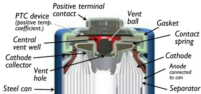
Close-up of the top part of an Energizer AA-size lithium battery showing safety features — PTC device and vent ball.
