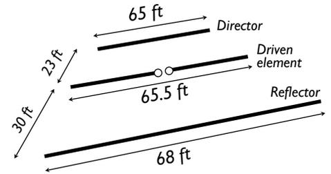
Dimensions of the 3-element sloping wire beam, viewed from behind the reflector.
