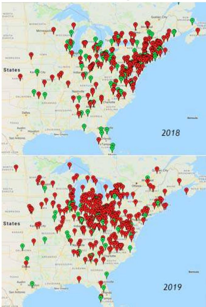
Distribution of 40 meter Field Day contacts using multi-band dipole in 2018 (top) compared with 40 meter wire beam in 2019. Red pin = phone, green pin = CW QSO. [Analysis courtesy Lou KD2ITZ and qsomap.org software.]
