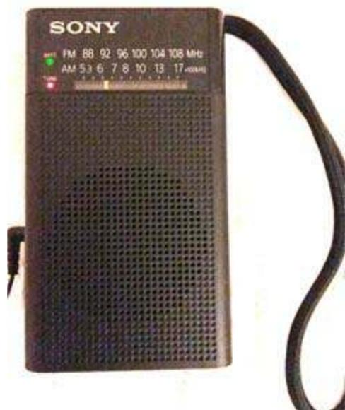
The Sony ICF-P26 AM/FM radio has a black enclosure, sized 4<sup>1</sup>/<sub>16</sub>" x 2<sup>3</sup>/<sub>4</sub>" x 1<sup>1</sup>/<sub>2</sub>". [N2KZ pic.]
