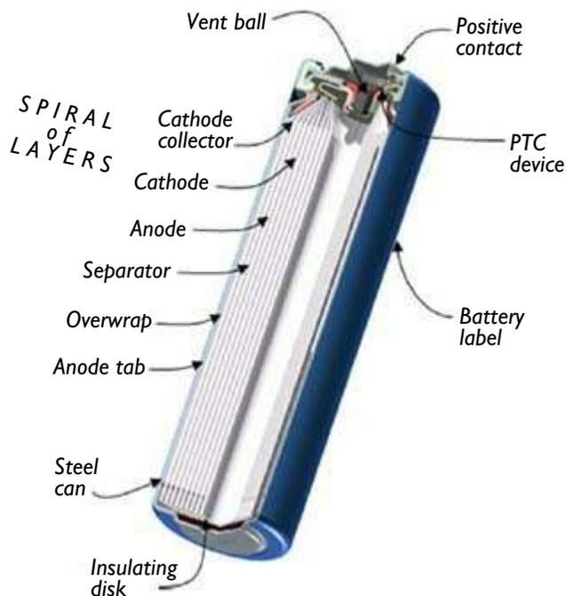
Diagram of an Energizer AA-size primary lithium battery based on  $\text{LiFeS}_2$  chemistry. The anode is made of lithium metal, the cathode consists of iron disulfide on an aluminum foil substrate. Electrolyte is a solution of lithium salts in an organic solvent. [After Energizer Brands.]
