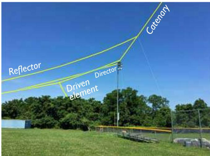
Fig 2. Wire beam antenna erected at the 2019 Field Day site. Wires and support ropes emphasized. [KD2ITZ pic.]
