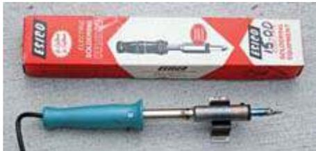
Esico 6150 150 watt soldering iron has large thermal mass in the tip.
