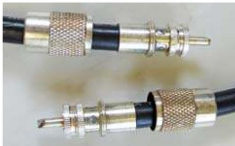
PL-259 connectors with **just enough** solder in the four solder holes to make a good bond between connector body and braid. Center conductor is soldered **inside** the center pin.
