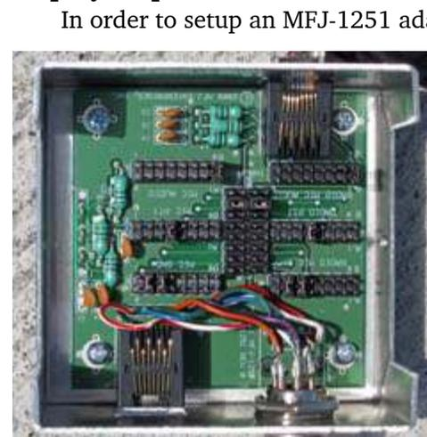
MFJ-1251 with modified jumper settings for an Icom 8-pin round microphone plug to an Icom 8-pin round MIC connector.
