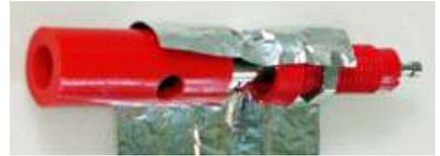
“Little better than a banana plug and socket with shielding wrapped around it.”
