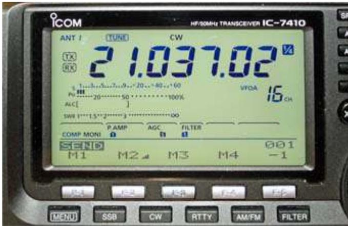
Icom IC-7410 display showing “MENU” key and function keys F-1 to F-5, ready to send from the four CW memories.
