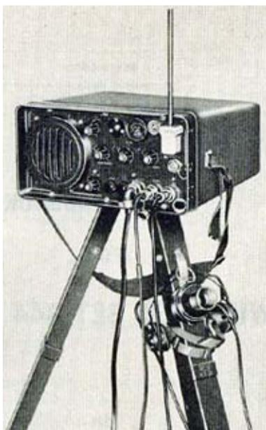
*B44 transceiver mounted on tripod for field use.*
