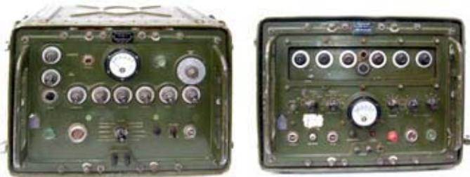
*Larkspur C41 transmitter and R-222 receiver for UK military communications. C41 wideband FM transmitter provided up to 35 watts RF output, 50-100 MHz.*
