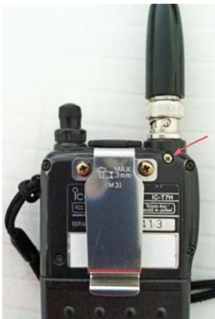
*Icom IC-T7H handi-talkie, with antenna screw arrowed in red.*
