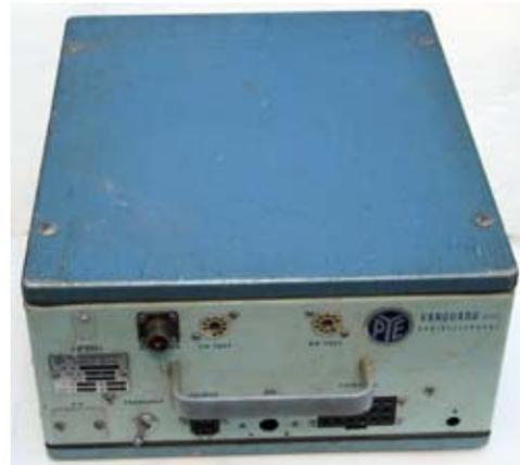
*Pye Vanguard AM25T transceiver used at G3VNQ, has 25 watts output.*
