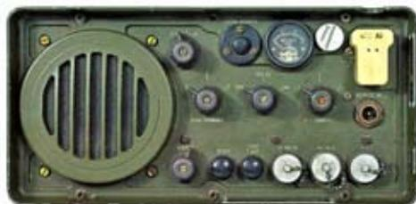
*B44 Mk III transceiver had three crystal-controlled AM channels in the range 60-95 MHz.*
