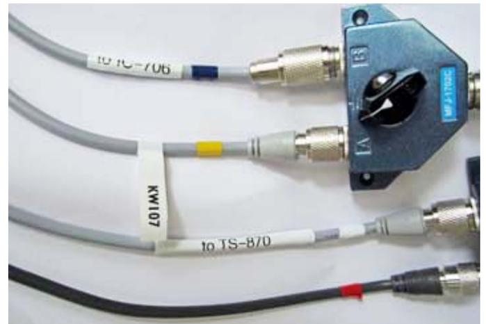
Labels for coaxial cables prepared with Brother's Flexible ID Tape. Lengthwise labels work best on wider cables (3/8 inch diameter and above).
