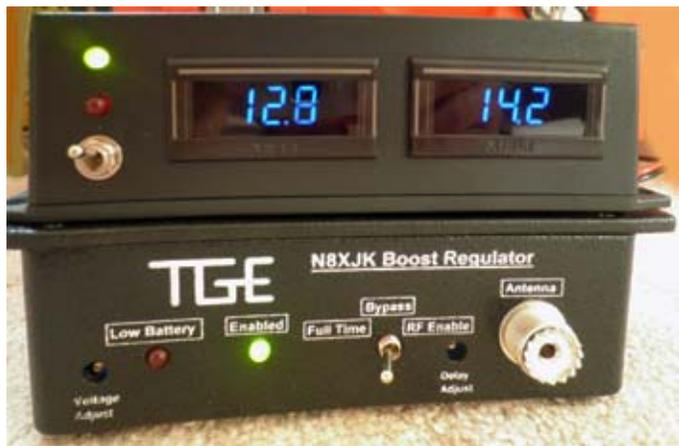
*TG Electronics' N8XJK Super Booster delivers up to 40 amps of regulated output. Ray's unit is shown with the matching TG Electronics Digital Remote Panel R-2 (top) which displays input and output voltage. [Photos W2CH]*
