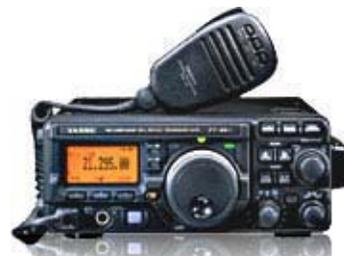
*Yaesu FT-897 HF/VHF/UHF transceiver is too small to have a front panel keypad.*
