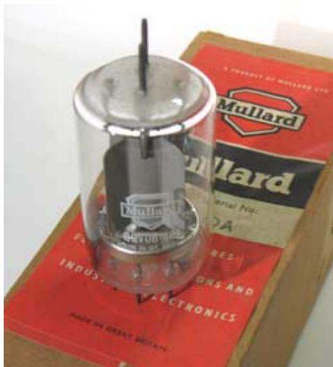
*Borosilicate glass is used in power tubes like this European QV06-40A (5894A) dual tetrode for VHF/UHF transmitters. The tube is internally neutralized and has the two separate anode connections brought through a tough, heat-resistant seal at the top of the glass envelope.*
