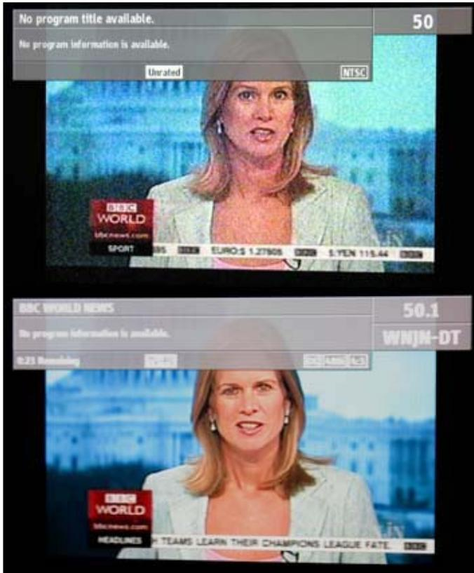
Comparison of over-the-air analog broadcast from WNJN (top) with standard definition 480i digital broadcast (bottom). While the analog signal on UHF channel 50 is noisy, the digital signal on WNJN-DT channel 51 (virtual channel 50.1) is noise-free. WNJN is located at Montclair State University.
