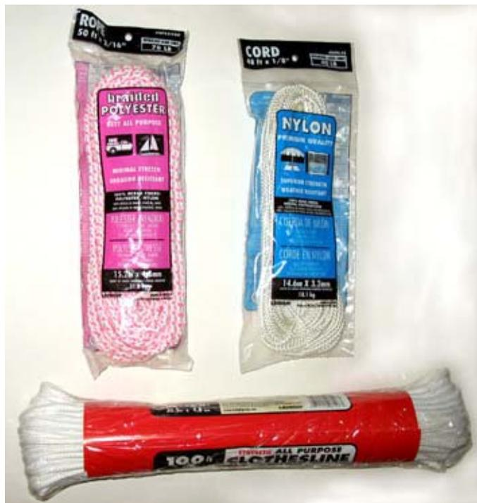
*The most suitable synthetic rope for raising antennas is polyester (top left). Nylon is stronger, but stretches too much. And while “poly” (polypropylene) rope is inexpensive and floats on water, it deteriorates in sunlight.*
