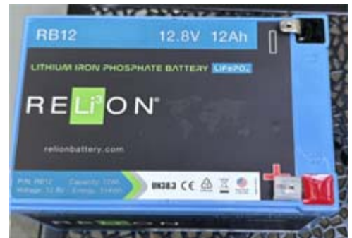
Top view of RELiON battery shows spade terminals at right. [KD2EVI pic.]
