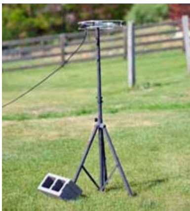
Low, omnidirectional VHF-FM antenna. [Credit: Nicholas Langan].
