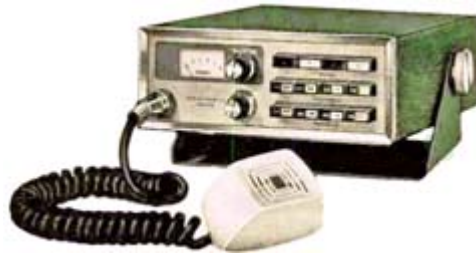
Heathkit HW-202 2 meter FM transceiver had six crystal-controlled channels.
