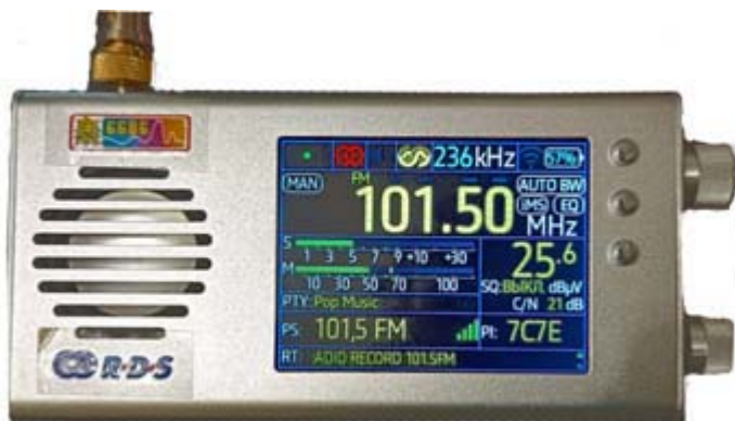
AM/FM radio receiver based on the TEF6686 single chip.
