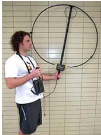
Portable magnetic loop antenna for 40 to 10 meters developed by Alex, PY1AHD.
