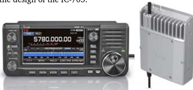
*Icom SHF-P1 controller (left) will be linked by Ethernet cable to a masthead RF module, with separate connections for 2.4 GHz, 5.6 GHz and GPS antennas.*
