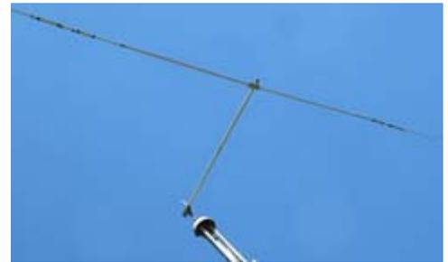
*One element was left up in the air after the boom of the tri-band beam fell apart.*
