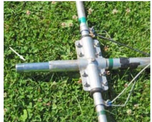
*Rich WZ2P inserted a length of threaded pipe (arrowed) into the boom at the point of separation.*
