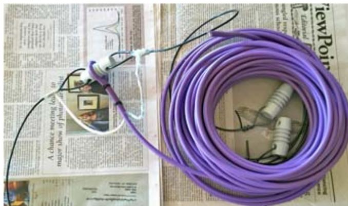
20 meter dipole fed with RG-6 type 75  $\Omega$  cable. [N2KZ pic.]
