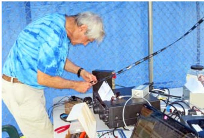
*Jay NE2Q prepares the 450 ohm ladder line feeder for connection to the 40 meter station.*
