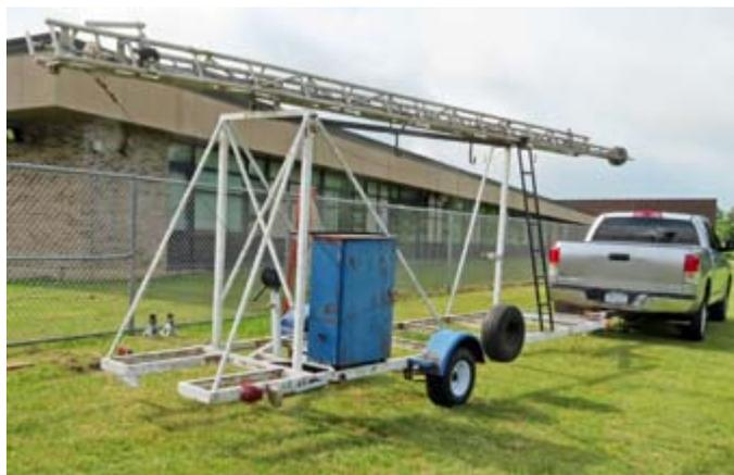
*The trailer with two-section tilt-over tower arrives on-site.*
