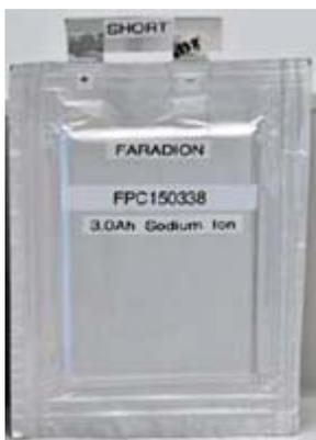
*Sodium-ion pouch cell by Faradion with terminals shorted.*
