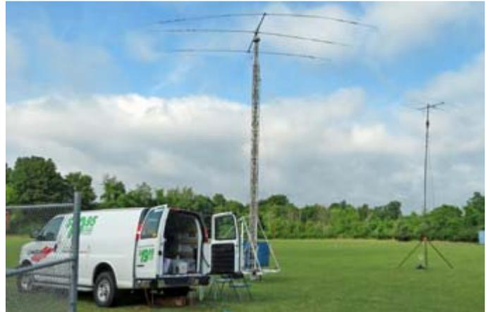
Field Day antennas included a tri-band beam mounted on the tower-trailer and a 6 meter beam (right).
