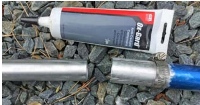
Pole ends after wire brushing to remove anodized surfaces, then coated with GB Ox-Gard antioxidant compound. Hose clamp is in position ready to hold the poles together.
