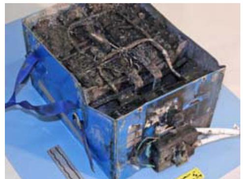
Charred lithium-ion battery from a Boeing 787 Dreamliner.
