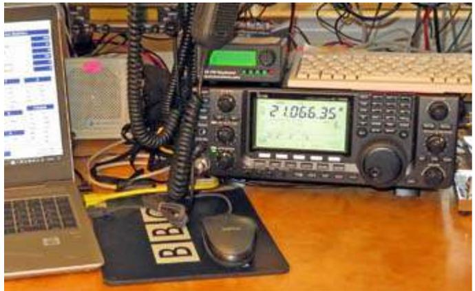
*The Field Day operating position at NM9J. Note the Hamcrafters K44 CW keyboard on top of the IC-7410.*
