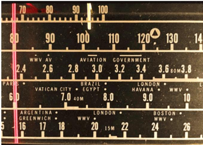
Tuning dial of Karl's Hallicrafters S-120 receiver, covering 0.55 - 1.6, 1.6 - 4.4, 4 - 12, and 11 - 30 MC\* in four bands, plus bandspread range, 0-100, at top. [N2KZ pics]
