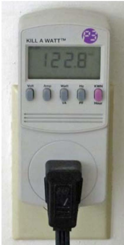
“Kill A Watt” indicates AC line voltage. For connected equipment, it can also show the current in amps, power in watts and power factor (VA).
