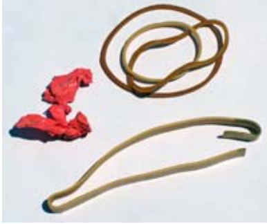
Natural rubber degrades with time. The red material was a rubber balloon. Old rubber bands break when stretched.
