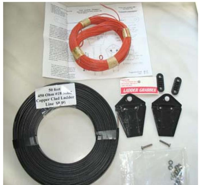
*Parts assembled for the home-brew ZS6BKW antenna include a reel of 450 ohm ladder line and an Emtech "Ladder Grabber".*
